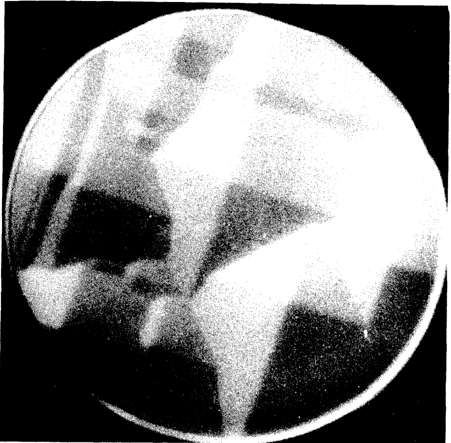
Fig. 5.49 A microphotograph of low pyramid formation during electrocrystallization of Ag on a single crystal Ag surface. (By courtesy of E. Budevski)
