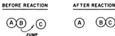
Fig. 4.38. A three-atom chemical reaction AB + C \rightarrow A + BC viewed as the jump of atom B from atom A to atom C .
