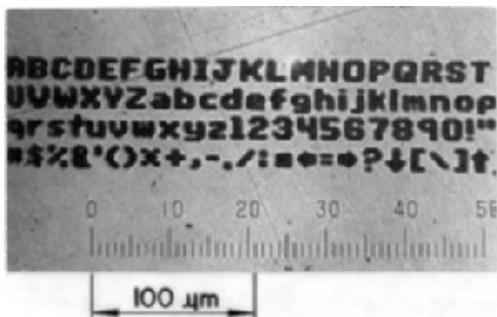
Figure 11. Photoelectrochemically etched character set in unbiased n^+ -GaAs using scanned 2\ \mu\text{m} diameter HeNe laser spot ( 160\ \text{W}/\text{cm}^2 , 0.2\ \text{sec}/\text{point} , 10\% \text{KOH} ) (24). Reprinted by permission of the publisher, The Electrochemical Society, Inc.
