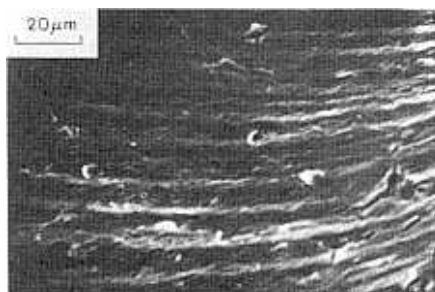
Figure 28. a) SEM photograph of SiC deposit on [0001] \alpha\text{-SiC} from melt of composition of 0.8 \text{Li}_2\text{CO}_3; 0.2 \text{SiO}_2 , using -0.5 volts vs. SiC. Deposition time, 3 hrs. b) SiC deposit under similar conditions to a) but at -0.4 volts for 30 mins (76).
