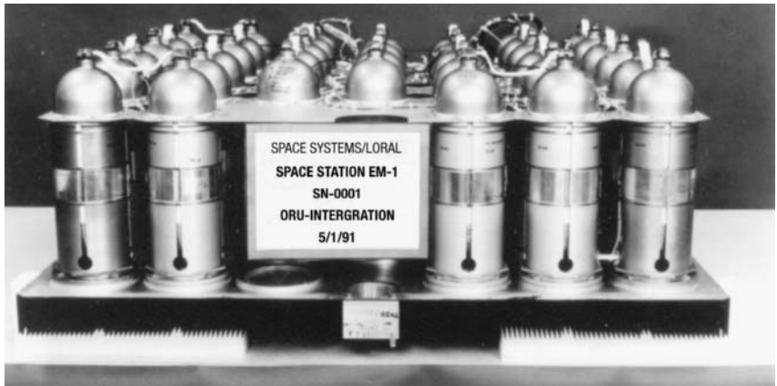
FIGURE 32.8 International Space Station 81-Ah Ni-H 2 38-cell assembly.
