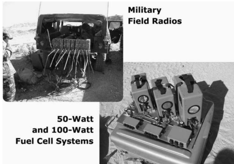
FIGURE 43.11 50-Watt and 100-Watt systems charging batteries of military field radios.
