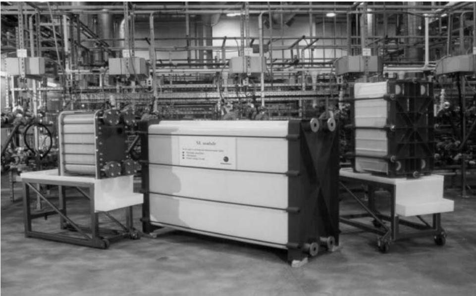
FIGURE 37.7 Regenesys modules of varying sizes. (From Ref. 25.)
