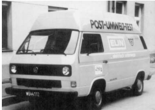
FIGURE 39.9 Volkswagon bus powered by SEA zinc/bromine battery. (Courtesy of SEA.)
