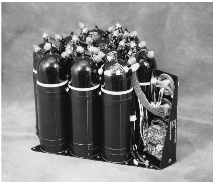
FIGURE 32.25 Mars Polar Lander 16-Ah CPV battery assembly.
