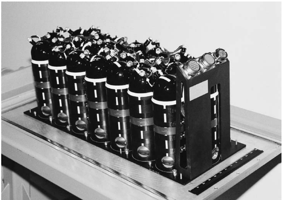
FIGURE 32.6 DMPS 100-Ah Ni-H 2 battery assembly.
