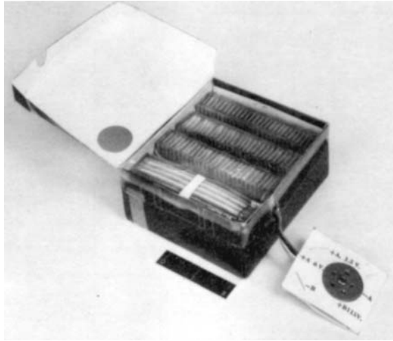
FIGURE 17.22 Magnesium/cuprous chloride radioisotope battery. Size: 10.2 \times 11.7 \times 1.9 cm; weight: 450 g, rated capacity: A 1 section—1.5 V, 0.3 Ah; A 2 section—6.0 V, 0.4 Ah; B section—115 V, 0.08 Ah.
