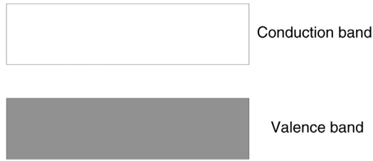
Figure 15.1 Illustration of energy bands formed in a crystalline solid.
