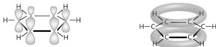
Figure 2.9.6 The structure of benzene: a The p orbitals before overlap (the sp^2 hybrids are shown by the straight lines); b The delocalised system of \pi bonds
