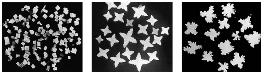
Figure 6.41. Habit changes in sodium chloride crystals caused by traces of impurity: (a) pure solution, (b) 0.1% \text{Fe}(\text{CN})_6^{4-} , (c) 1% \text{Fe}(\text{CN})_6^{4-} . (Cooke, 1966)
