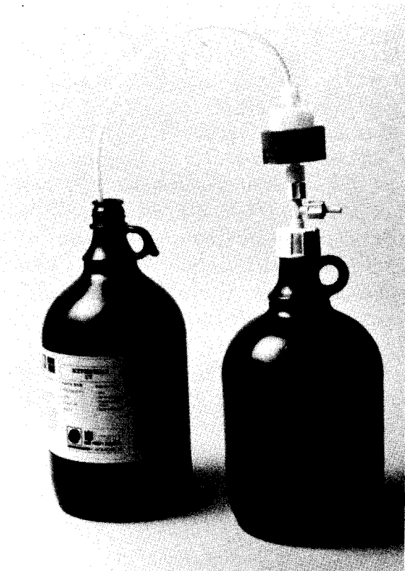
Fig. 6.9. Filter-degasser apparatus allows vacuum filtration of mobile phase directly into reservoir. Courtesy of Lazar Research Laboratories.
