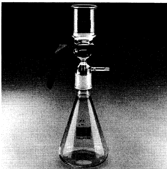
Fig. 6.11. Solvent filtration kit: Filter is placed on a stainless-steel screen at (a), clamped to the funnel cup (b), and fitted to a vacuum flask via a ground-glass joint. Courtesy of Millipore Corporation.
