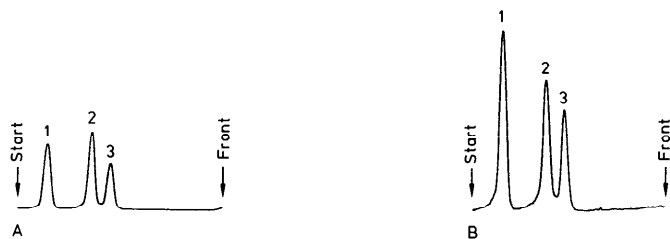
Fig. 2: Reflectance scan (A) and fluorescence scan (B) of a chromatogram track with 1 \mu\text{g} (A) or 200 ng (B) each substance per chromatogram zone: 1 = estriol, 2 = estradiol, 3 = estrone.
