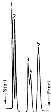
Fig. 1: Reflectance scan of a chromatogram track with 300 ng substance per chromatogram zone: 1 = azinphos methyl, 2 = azinphos ethyl, 3 = parathion methyl, 4 = fenitrothion, 5 = parathion ethyl + phoxim.
