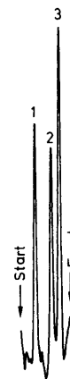
Fig. 2: Reflectance scan of a chromatogram track with 500 ng azinphos ethyl (1), 580 ng malathion (2) and 590 ng diazinone (3) per chromatogram zone.
