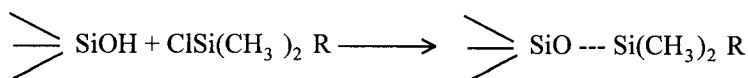
Figure 2.3 Reaction of silica gel with a functional group to produce a reversed-phase stationary phase.
