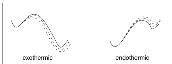
Fig. 3.9. Energy profiles for series of related reactions illustrating the Bell-Evans-Polyani relationship.
