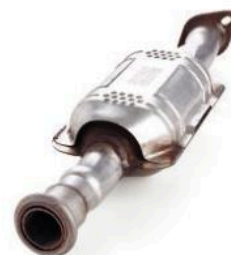
▲ A catalytic converter. This changes harmful car exhaust gases into less harmful ones.
