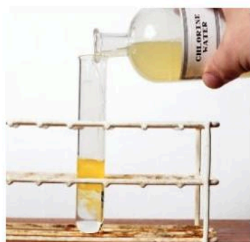
◀ Chlorine solution reacting with potassium bromide solution.
