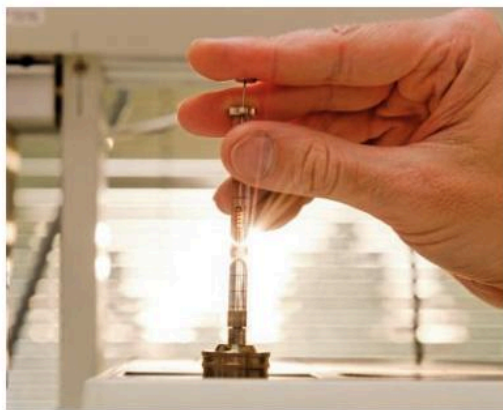
▲ Injecting a sample for gas chromatography.
