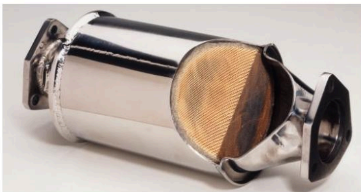
▲ The honeycomb structure of a catalytic converter.
