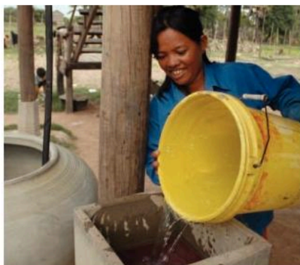
▲ Sand filtration helps make water safe to drink.
