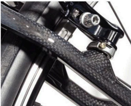
▲ Part of a carbon-fibre-reinforced plastic bicycle frame.
