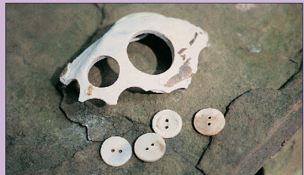
BOX FIGURE 3 Shell of a freshwater mussel after having been drilled to make pearl buttons.
