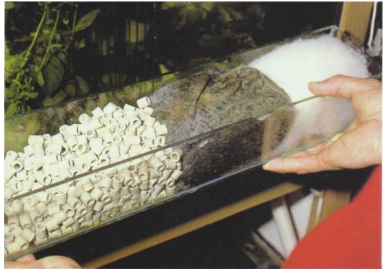
Gutter filter equipped with thick filtering media (left) and finer ones (right). V
