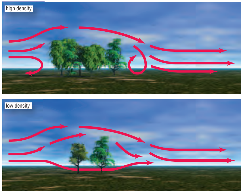
How a shelter belt works
