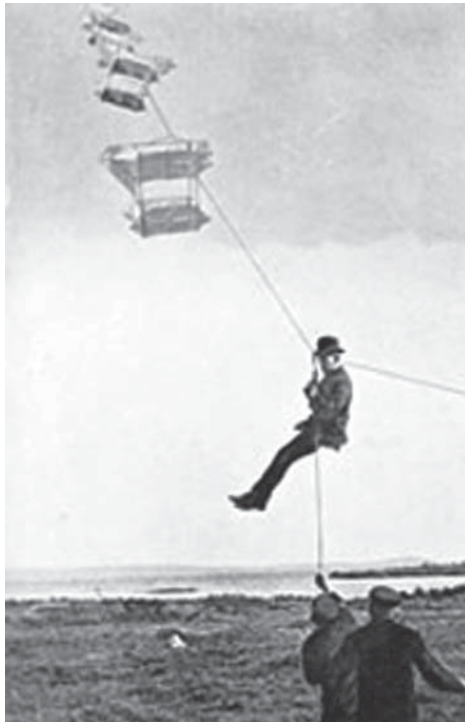
Polar explorer Roald Amundsen takes flight using a chain of man-lifting kites during experiments in 1909.
