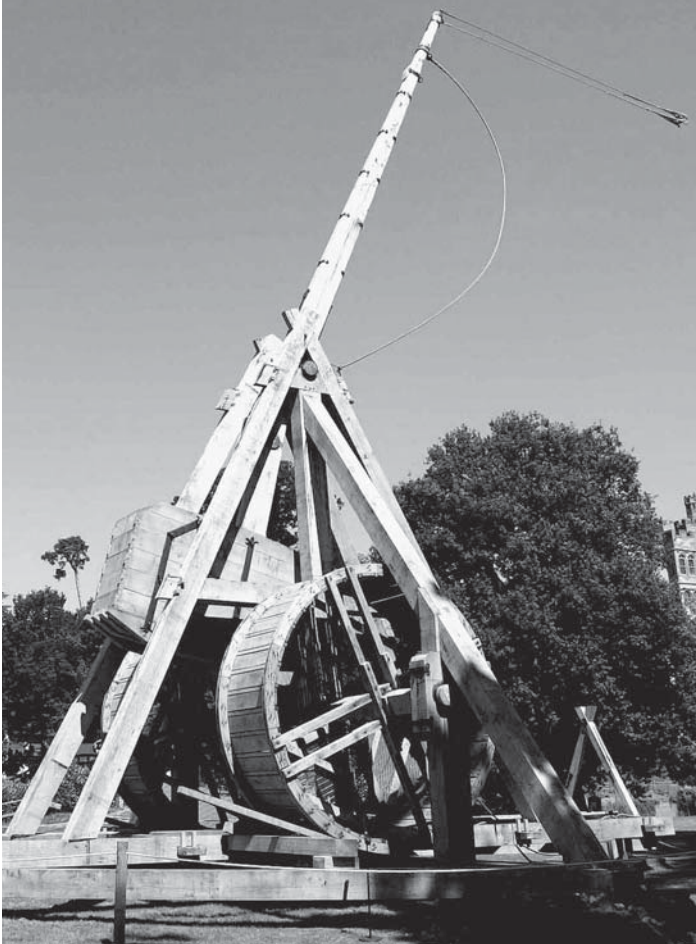
The Warwick Castle trebuchet in action. The thirty-three-ton machine—the largest working trebuchet today—can launch a thirty-pound payload nearly a fifth of a mile.
