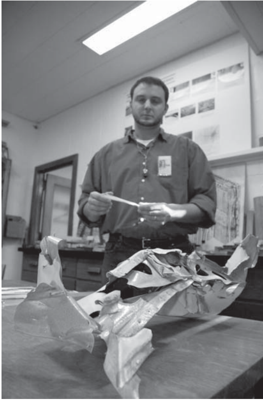
Alex Wiedenhoef of the Forest Products Laboratory stands behind a crumpled section of a small plane, holding a fragment of the wood propeller that helped determine the cause of the accident.
