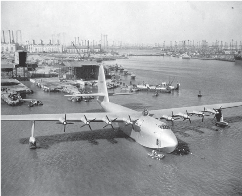
The Spruce Goose floating on water. Despite its nickname, the Spruce Goose was a mere 5 percent spruce. The largest aircraft of its day, built primarily by woodworkers and paper hangers, it weighed 400,000 pounds, stood eight stories tall, and had eight propellers, each 17 feet in diameter.
