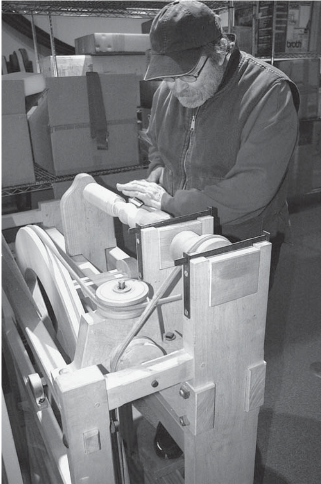
Alan Lacer test-drives a replica of an early wooden treadle lathe. The tools of his trade date back to at least 800 BC.
