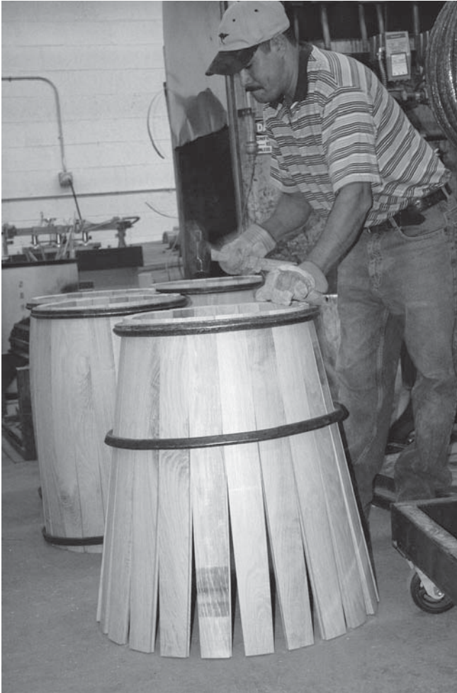
Raising rings are used to hold staves together temporarily during the first stages of barrel building. The process uses a blend of hundred-year-old cast-iron contraptions, computer-guided machines, hand labor, and mechanization.
