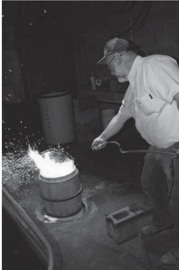
Fire bursts from the top of a sawdust-filled oak barrel as Russ Karasch of the Barrel Mill adds compressed oxygen to fan the flames. The charred barrel will be used to age whiskey for three to eighteen years; then it will be shipped overseas (or be turned into a driveway planter).
