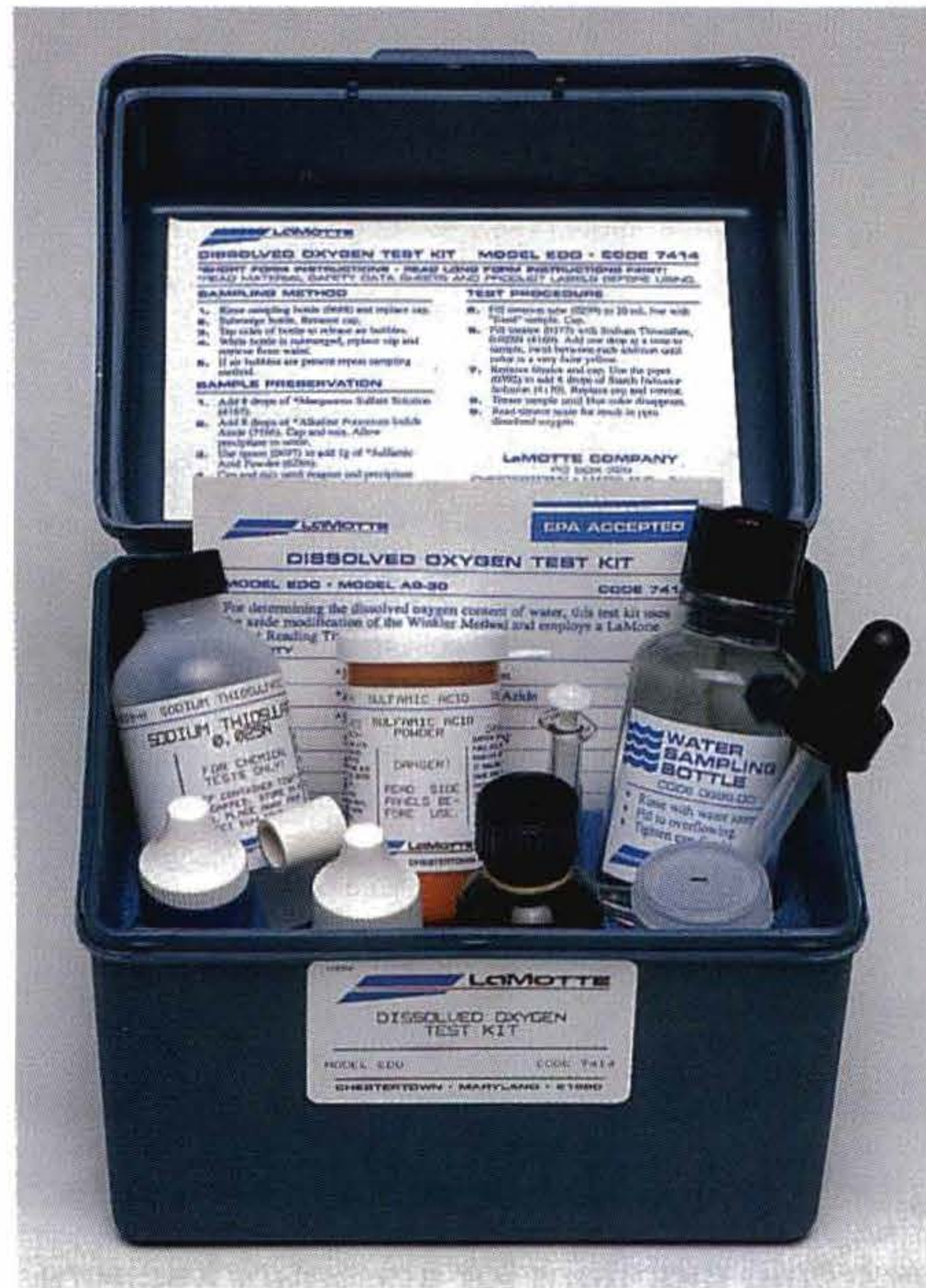
Dissolved oxygen test kits, one of many diagnostic tools for advanced aquarists.
