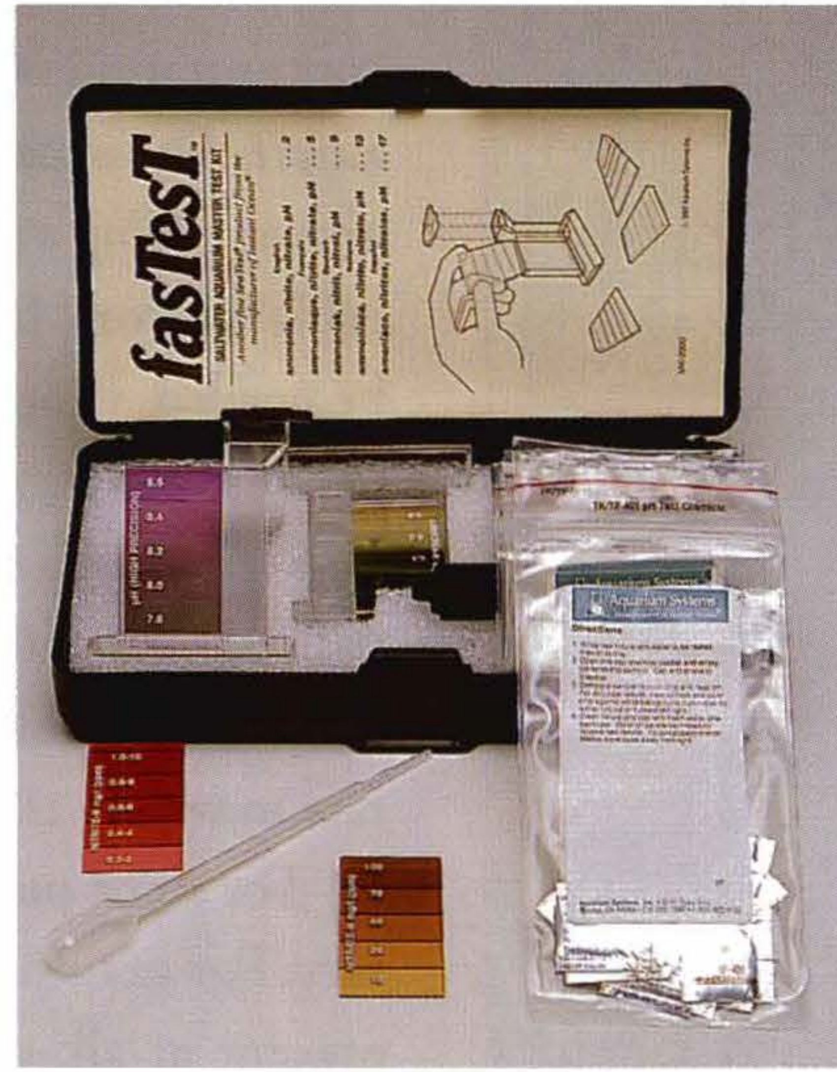
A basic marine test kit to check levels of ammonia, nitrite, nitrate, and pH.
