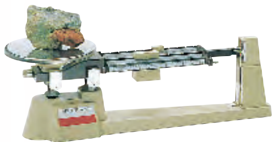
Figure 12 A triple-beam balance is used to determine the mass of an object.
