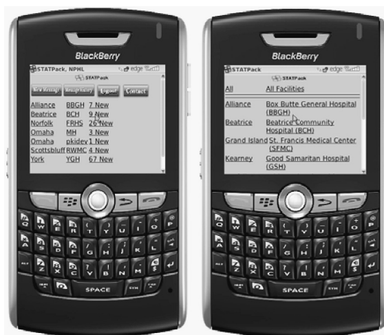
FIGURE 17.5 Mobile facilities screen. STATPack mobile provides an additional screen, which displays only the new messages. The user can opt to view just the new messages or can view the complete list of messages by clicking on the Message History button.
