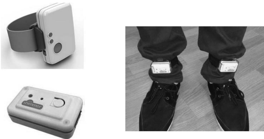
FIGURE 25.16 Wrist and ankle sensors and kinematic measurement setup with a wireless sensor network.
