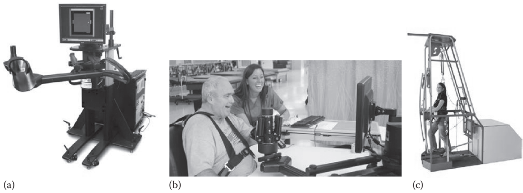
FIGURE 1.7 Examples of end-effector-based system for rehabilitation: (a) InMotion ARM (Interactive Motion Technologies), (b) InMotion HAND (Interactive Motion Technologies), and (c) Gait Trainer GT I (Reha-Stim). (Courtesy of Interactive Motion Technologies, Watertown, Massachusetts, and Reha-Stim, Berlin, Germany.)
