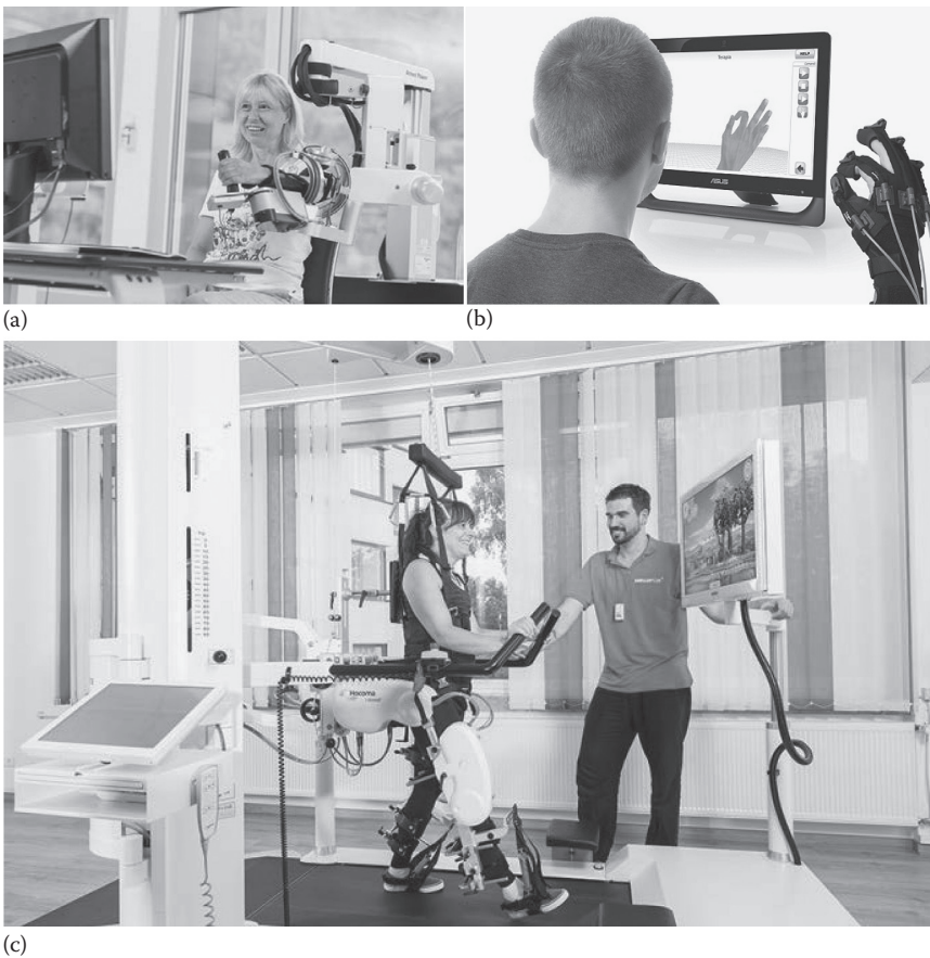
FIGURE 1.8 Examples of exoskeleton type devices for rehabilitation: (a) Armeo®Power (picture: Hocoma, Switzerland), (b) GloReha (picture: Idrogenet, Italy), and (c) Lokomat (picture: Hocoma, Switzerland).
