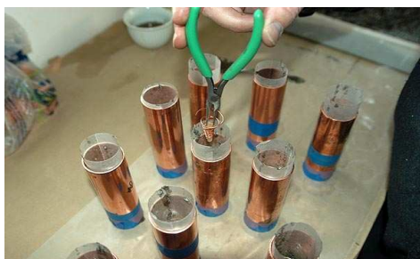
Earth pipes in the making
