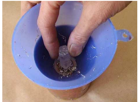
Place top crystal into nest with tip facing downward (up in finished HHG)
