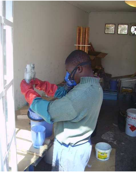
Measure needed quantity of catalyst
