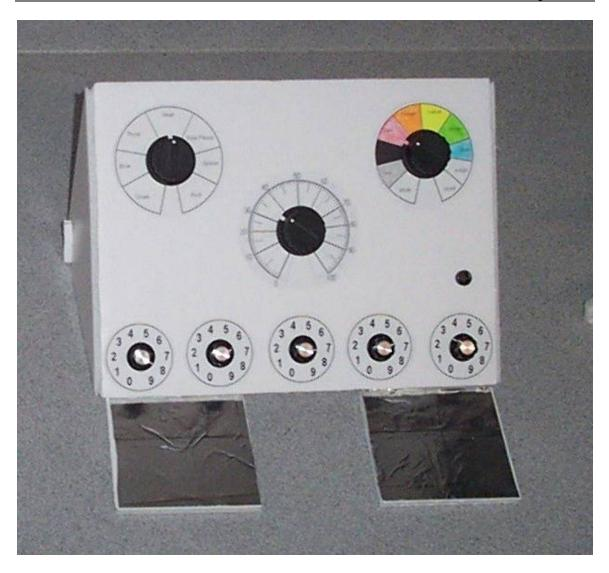
This machine was designed in a way to keep its construction as simple as possible so that it can be built by anyone. Therefore I decided to use poster board for its construction since it's much easier to work with than wood or metal. In fact no power tools are even needed except for a soldering iron which can be purchased at radio shack for around \$7 if you don't already have one.
