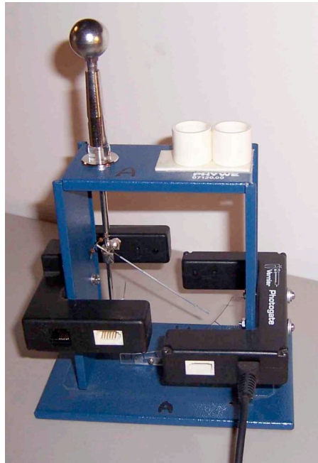
Kolbe-type Elecroscope, with Vernier Photogates. Used for precision measurement of the time of spontaneous discharge
