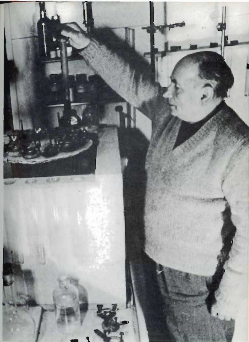
Putting the test-tubes into a circular oven with twelve apertures. The test-tubes are heated for four hours, then left to stand for four hours. This process is repeated seven times. The tops of the test-tubes protrude from the oven, assisting condensation of the vapours and regulating the pressure in the tubes.
