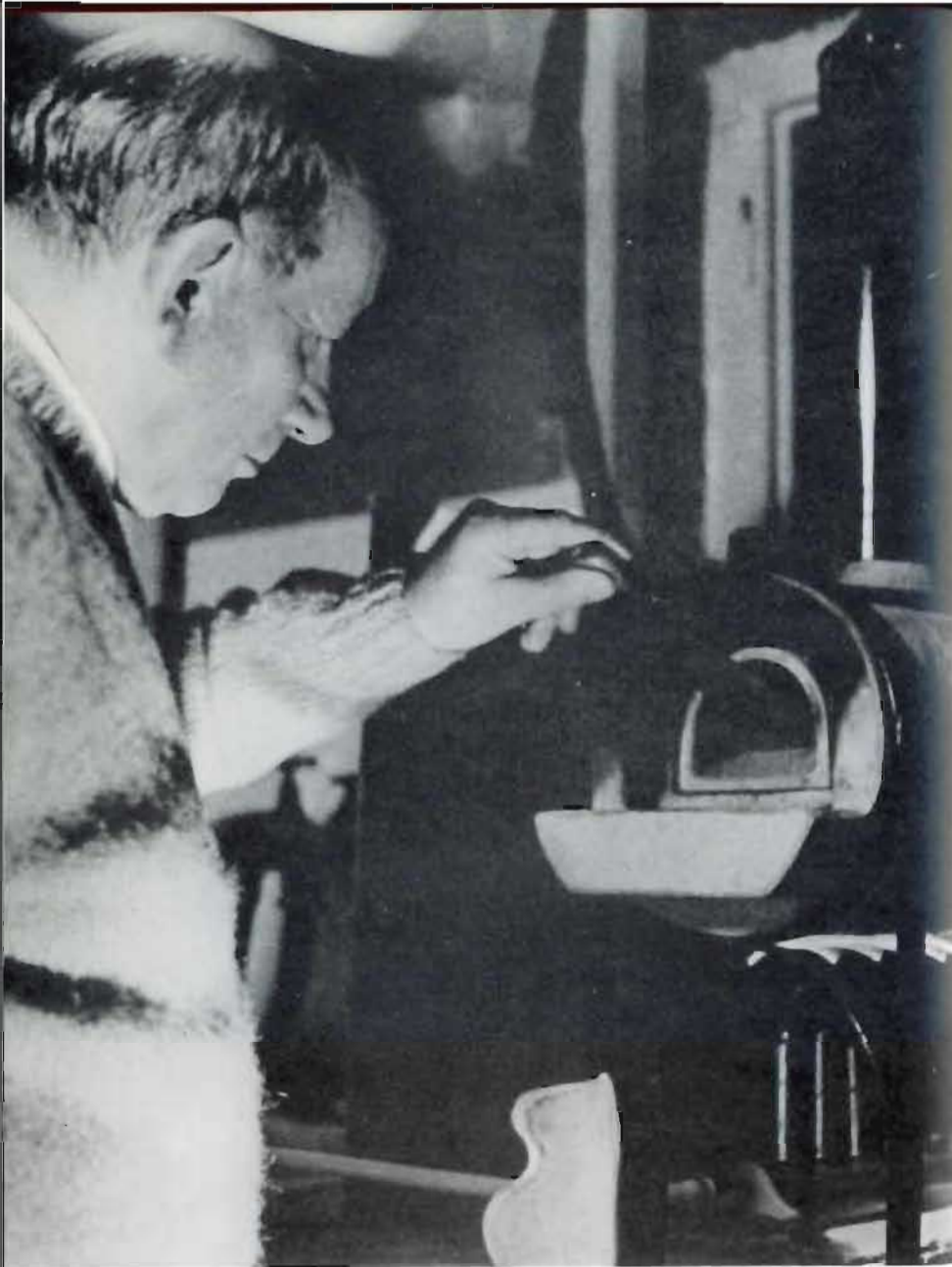
Incineration. Once the peat is fully dried out it is freed from any remaining deposits of carbon by incinerating it in an oven at a temperature of between 700 and 800°C. This operation takes several hours. Thus are obtained the ashes containing the vegetable salts.
