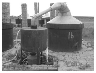
**FIGURE 5.2** A single distillation unit in Anhui Province showing the condenser tank which houses a spiral tube condenser and receiver.
