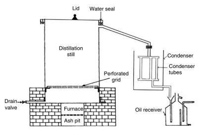
**FIGURE 4.7** The design of the steam-cum-water distillation equipment fabricated locally in the mint villages for the distillation of mint herbage in small batches.
