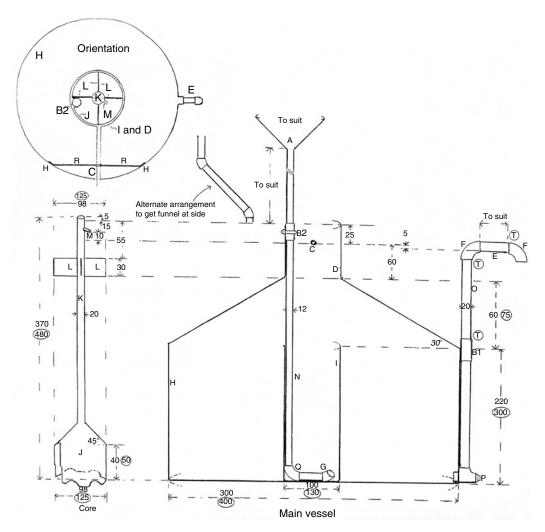
**FIGURE 6.14** Schematic representation of a distillate receiver–separator for mint oil. This is a compact design to be used with pilot stills (Figure 6.12) with a distillate flow of 40 L/h. Core is inserted down the neck of the main cylinder to rest on the base (floor) of the inner cylinder.
