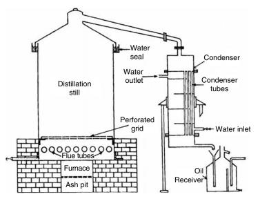
FIGURE 4.8 The structure of a high-efficiency distillation unit for batch-wise distillation of mint herbage designed by CIMAP, Lucknow, India.
