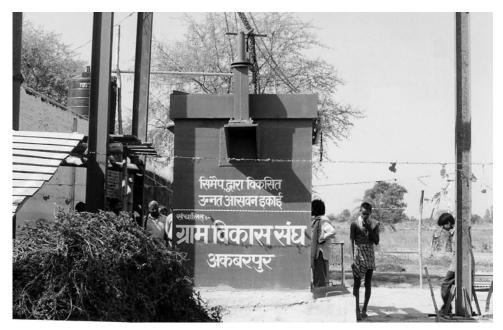
**FIGURE 4.12** Mint herbage distillation unit designed by CIMAP, Lucknow, installed for cooperative use in a village in Barabanki district of Uttar Pradesh in India.
