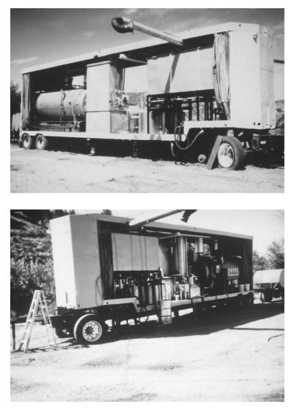
FIGURE 6.6 Example of mobile distillery designed by Newhouse Manufacturing, Inc.
