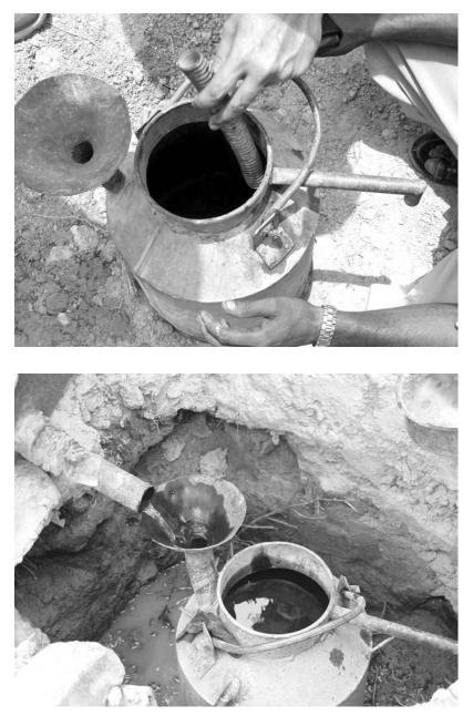
FIGURE 6.8 The converted milk can receiver (oil separator) used in India.
