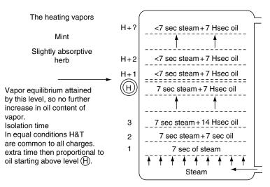
**FIGURE 6.15** Hypothetical schematic representation of steam or oil movement throughout the charge during steam distillation (H = charge height; T = time).
