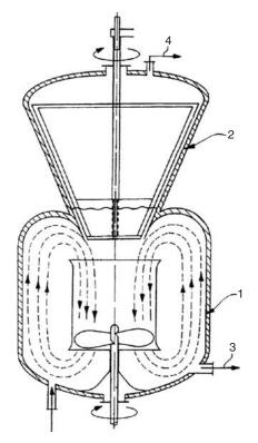
FIGURE 10.12 Crystallizer for the separation of (-)-or (+)-menthyl benzoate (Figure 5 in EP 909–205).
