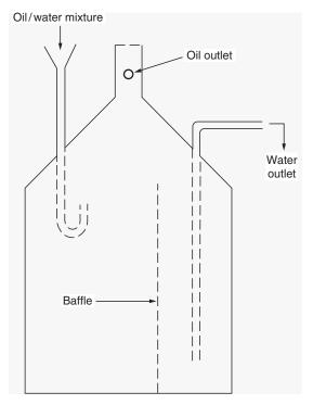
FIGURE 6.9 Modified oil separator designed by CIMAP.
