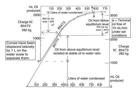
**FIGURE 6.16** Graphical representation of the distillation of two mint charges with different heights and top areas. The temperature gradient and vapor composition equilibrium occur during initial heating at a level below the top of the charge.
