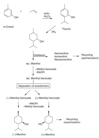
FIGURE 10.11 Total synthesis of (-)-menthol from m-cresol: The Haarmann and Reimer process.
