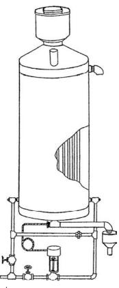
**FIGURE 6.3** Vertical condenser of  $5\frac{1}{2}$  ft (1.68 m) height and 28 in. (71 cm) diameter fitted with a large built-in vent to prevent pressure buildup, designed for use with an automatic water control valve and mint oil separator (receiving can) used in the 1960s.
