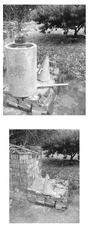
FIGURE 6.10 Unusual condenser system and commonly used receiving can (oil separator) used in cornmint oil distillation in China.
