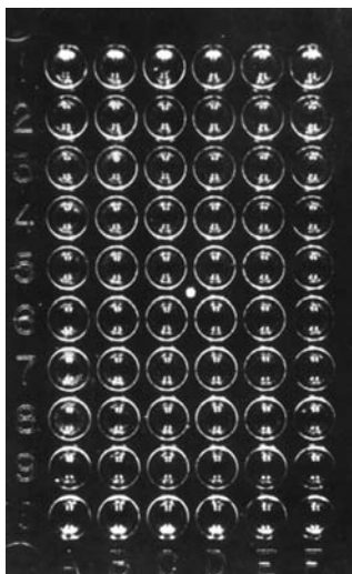
A Terasaki plate consisting of depressions in a plastic plate that contains pre-dispensed antibodies to HLA antigens of various specificities and into which are placed patient lymphocytes and rabbit complement for tissue typing.
