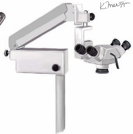
Operating microscope with three sets of binocular eyepieces for operator, 1st assistant, and 2nd assistant or television camera
