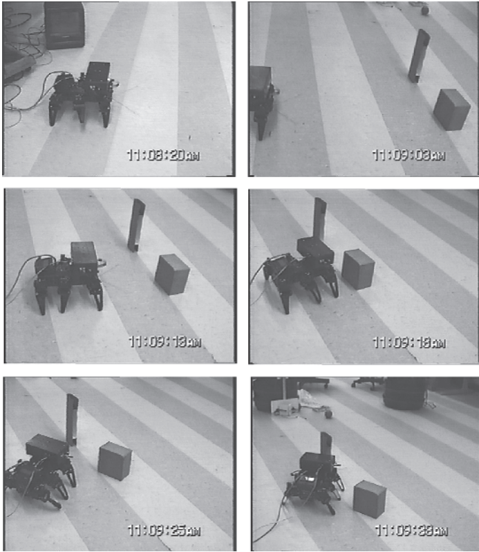
Figure 9.3. Top photos: The robot is initially still due to a high fear level as a predator object is in view off to the right. Middle photos: Once the predator object is removed, the robot moves toward a prey object to satisfy its hunger. Bottom photos: Once its appetite has been satisfied, it ignores the food object and moves toward the tall object, which represents a mate.
