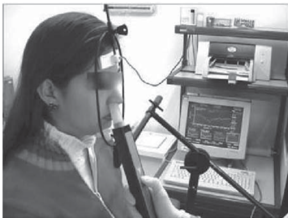
Figure 2.15 Picture of a computerized acoustic rhinometer system. The long vertical tube is attached to one nostril. The sound waves sent into the nose via this tube are reflected back into the same tube and analyzed by computer. (Figure reproduced with permission from the Scientific Electronic Library Online (SciELO) Brazil.)
