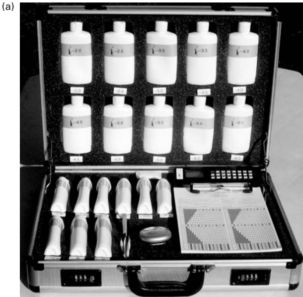
Figure 2.6a Examples of two commercially available threshold test kits. (a) The Smell Threshold Test (STT; Sensonics Inc, Haddon Hts., NJ, USA). The rose-like CN I stimulant, phenyl ethyl alcohol, is provided in 17 half-log concentration steps ranging from -10 log vol/vol to -2 log vol/vol. The stimulus is delivered with squeeze bottles and a single staircase method is used to present the stimuli – see Figure 2.7.
