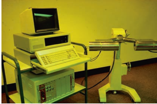
Fig. 12.1 Dual detector system for measuring positron-emitting tracers in the brain.
