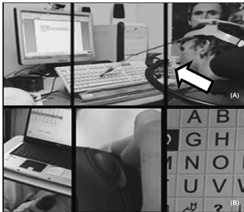
FIGURE 12.2 Communication systems via small movements. (A) A chin-contactor (white arrow) allows the LIS patient to control his wheelchair and a head mounted contactor allows him to use an adapted personal computer; (B) finger-controlled text-to-speech synthesizer. Source: Taken from Bruno et al. (2009).
