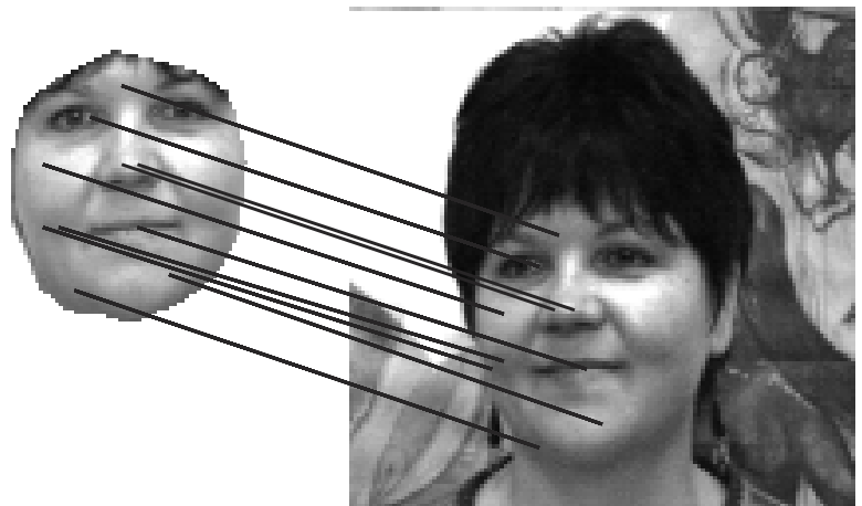
Figure 1. Correspondence maps provide a basis for a similarity measure between two facial images, which is used for person identification. They also deliver information about pose, size, and expression, and are crucial for animation. Their computation is difficult and rarely perfect. The figure shows selected correspondences obtained with the algorithm from Würtz (1997).
