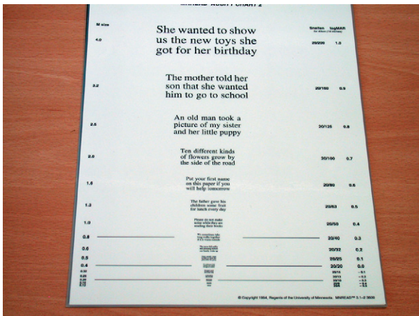
Figure 1.3 The MNRead is an example of a near logMAR chart
