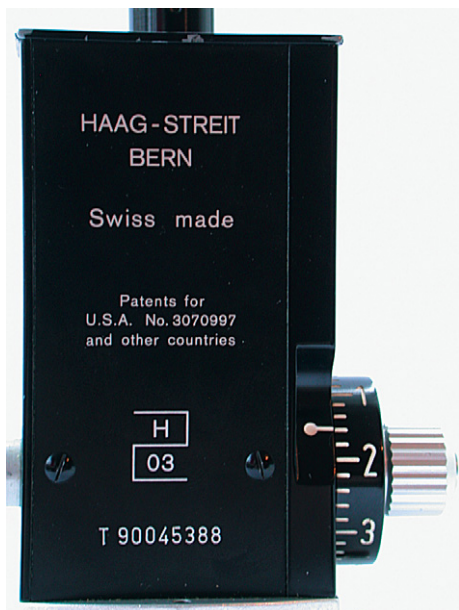
Figure 6.3 Goldman tonometer. Note calibration is in grams
