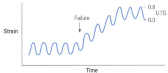
Figure 7.11 Fatigue failure. When a force of constant peak magnitude is applied cyclically, the material initially deforms repeatedly to the same extent, but at some point the strain increases even though the load has not changed. This point indicates the onset of fatigue failure. UTS, ultimate tensile stress.
