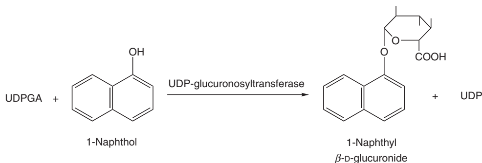
Figure 9 Conversion of 1-naphthol to its corresponding \beta -D-glucuronide.
