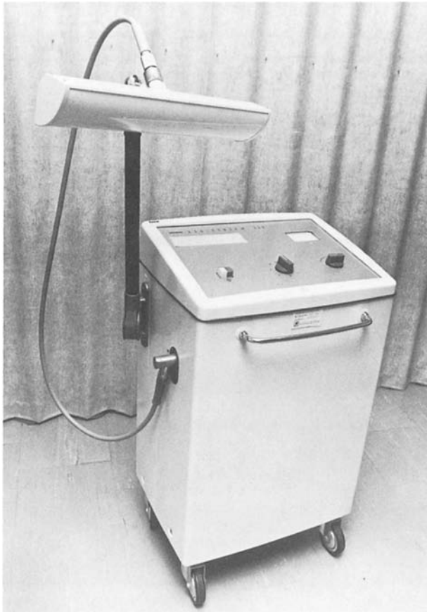
Figure 9. Microwave diathermy equipment. The microwave generator contains a magnetron that produces high frequency alternating current. This current is carried by a coaxial cable shown on the left to a transducer (upper left) containing an antenna and a reflector. The antenna converts the electric current into microwaves that are collected by the reflector. This focuses them and beams them into the body, where they are transduced into heat.
