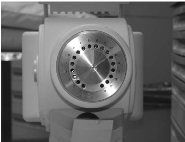
Figure 8. The frontal view of an indexer from the Nucletron, MicroSelectron HDR RAL, consisting of 18 channels.
