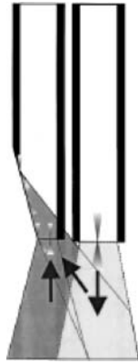
Figure 14. Design of the fiber tip of a typical fiber optic probe for Raman spectroscopy (62).
