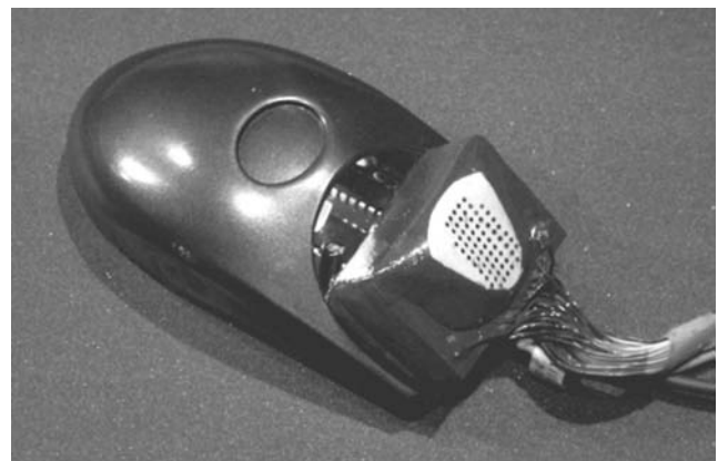
Figure 6. Mouse-mounted tactile display. Mouse-mounted tactile display with 64 electrodes. The stimulating current is controlled by a force sensor located under the electrodes, allowing the user to control stimulus intensity and reducing frequency of painful shocks. (Photo provided by Hiroyuki Kajimoto.)
