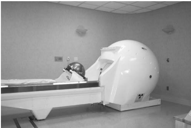
Figure 1. The Leksell Gamma Unit Model U for treatment of patients with brain tumors and other brain abnormalities.
