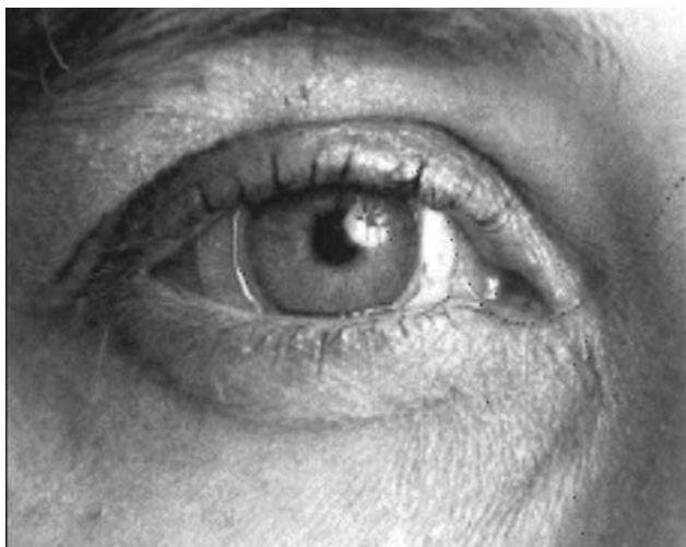
Figure 5. An annular search-coil contact lens used to measure the horizontal and vertical eye movements of a human subject. The fine wire from the imbedded coil exits at the nasal canthus.
