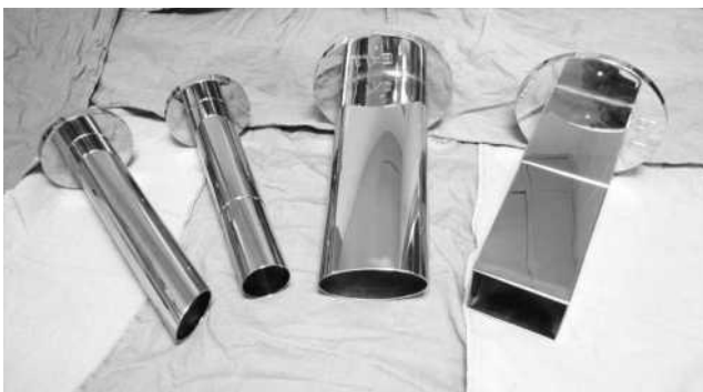
Figure 10. Examples of metal cones used in electron IORT. From left to right are shown a circular with bevel, a circular, an elliptical, and a rectangular applicator.
