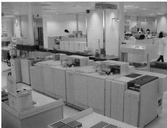
Figure 2. The Roche/Hitachi Modular™ analytic system has a theoretical throughput of 3500–5000 tests or 150–250 samples/h. They test 24 different analytes simultaneously with a total menu of > 140 available tests.
