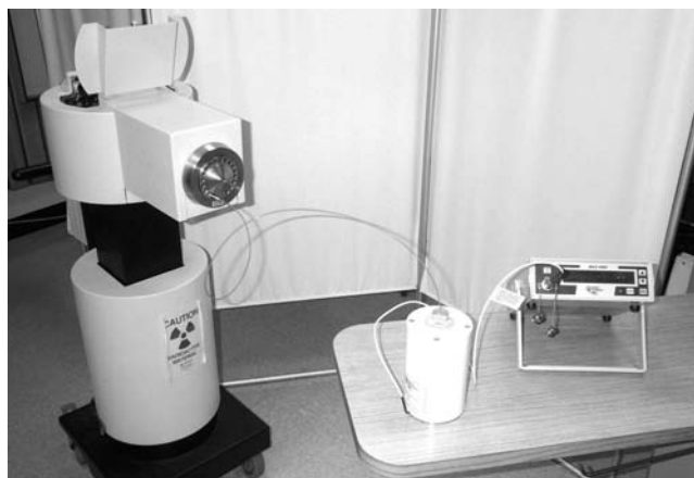
Figure 17. View of the HDR system with one catheter hooked up to a well chamber for calibration of the source by a medical physicist.
