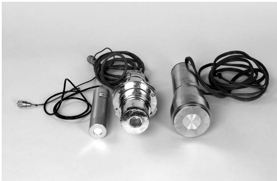
Figure 10. The NaI(Tl) detectors: 1 × 1 in. (left; Cardinal Health; Inovision, Model 425-110); 2 × 2 in. (5.08 cm) with center well (center; Nuclear Chicago, Model 321330), and 3 × 3 in. (2.62 cm) (right; Picker Nuclear Omniprobe, Model 2830-A).
