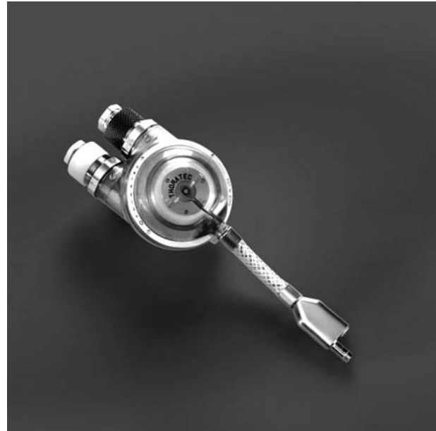
Figure 2. Penn State/Thoratec Pneumatic Ventricular Assist Device. The ventricle contains a flexible blood sac made of segmented polyurethane that is housed within a rigid polysulfone case. Mechanical heart valves are located in the inlet and outlet positions of the ventricle to control flow direction. Air pulses that are generated by an external drive unit are used to periodically compress the flexible blood sac. (Reprinted with permission from Thoratec Corporation.)
