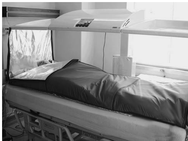
Figure 2. Heckel HT-2000 radiant heat whole body hyperthermia system. Unit at the University of Texas Medical School at Houston. Patient is in the heat maintenance phase of treatment, wrapped in the thermal blankets which form the sides of the chamber during active heating.
