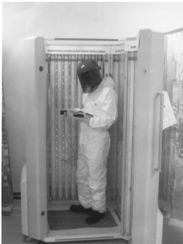
Figure 14. A common type of whole body phototherapy therapy supplied by Waldmann (Herbert Waldmann GmbH & Co., Villingen-Schwenningen, Germany.) This illustrates the direct method of measuring UV irradiance; after the door is closed lamps are lit and measurements are made in a number of positions.
