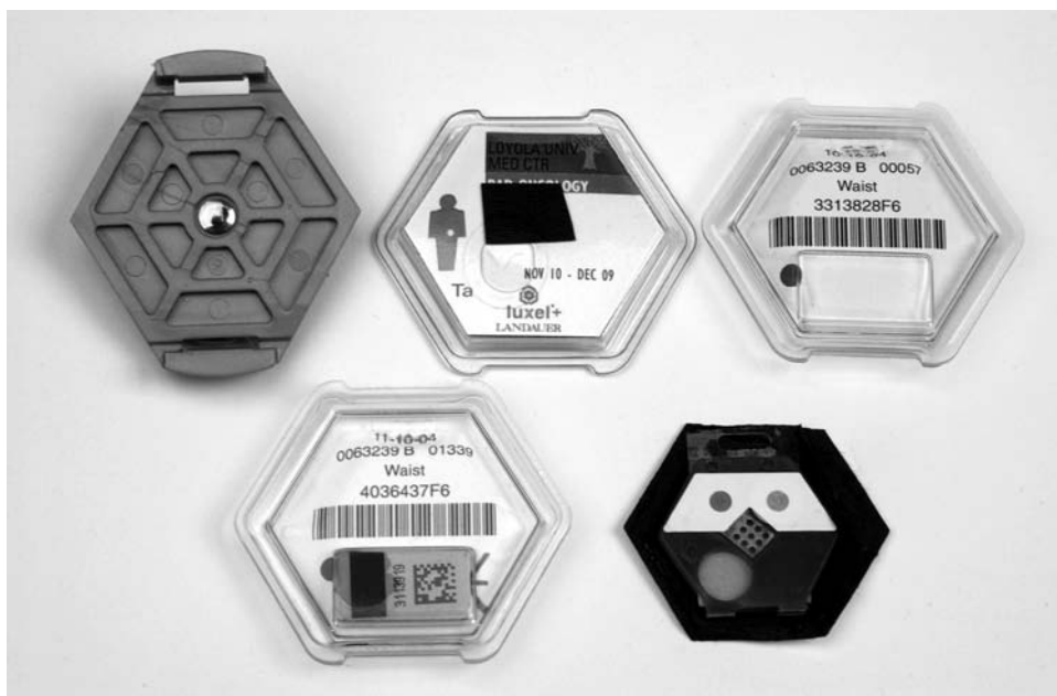
Figure 17. The Luxel Dosimeter: Holder (top left); front view (top center); rear view (top right); rear view with attached Neutron 144 detector (bottom left); detector element showing Cu filter (right), the Al filter (left), and plastic filter (circle, lower center). (Courtesy Landauer, Inc.)
