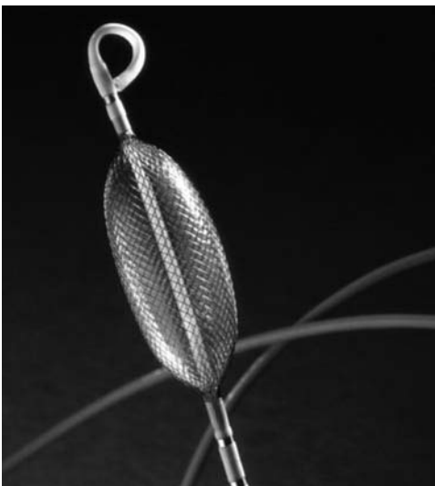
Figure 20. Ensite array catheter has 64 electrodes located on the surface of an expandable balloon catheter. The catheter records signals while floating inside the heart without contact. (Image provided courtesy of Endocardial Solutions.)
