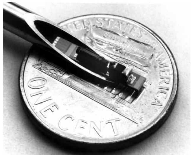
Figure 12. Photograph of the microstimulator in the bore of a gage 10 hypodermic needle.
