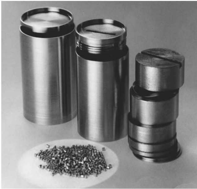
Figure 3. Cobalt pellets and source capsule with components.
