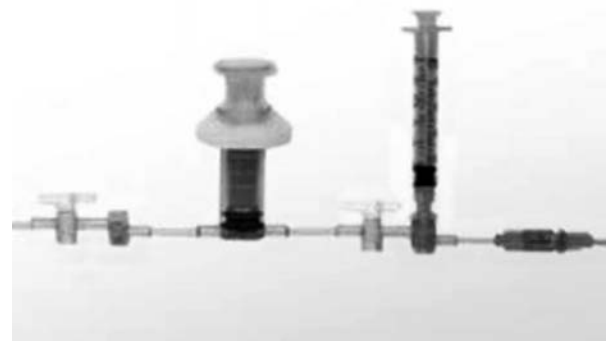
Figure 5. Diagram of the VIA LVM in-line ex vivo monitor and its components at the neonate bedside.
