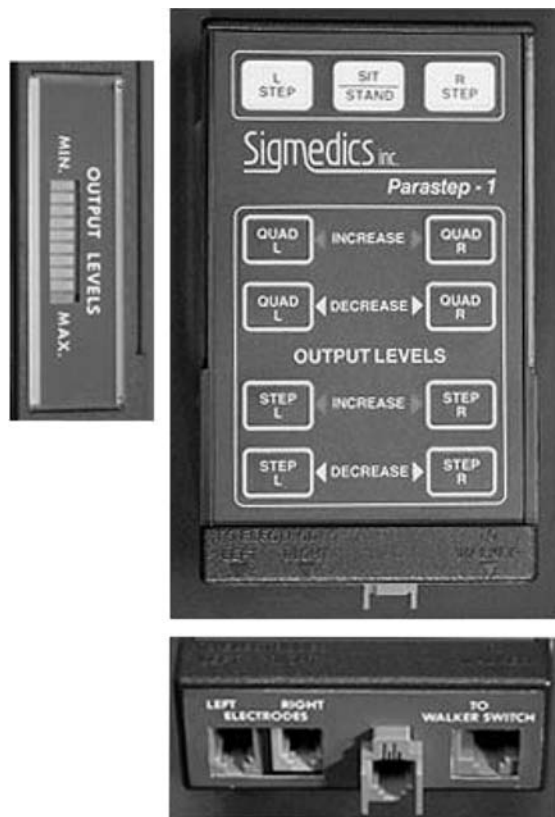
Figure 5. The neuromuscular stimulation unit for the Parastep system manufactured by Sigmedics, Inc. is battery-powered and microcomputer controlled. Cables connect the unit to surface electrodes, as well as to finger activated control switches on a walker. (Courtesy of Sigmedics, Inc.)
