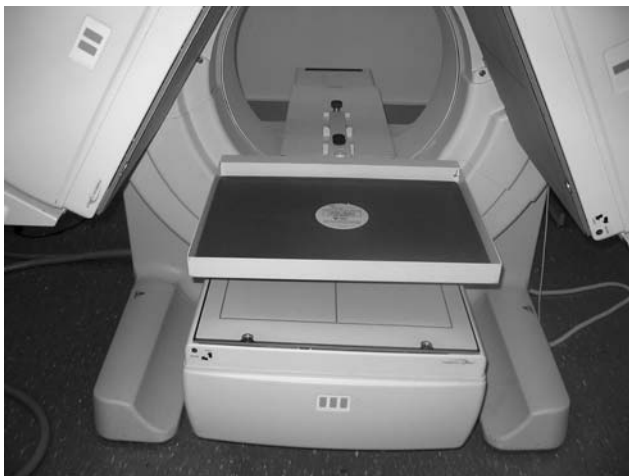
Figure 9. Radioactive sheet source in front of the third head of a three-headed SPECT system in position for checking uniformity and loading correction factors.
