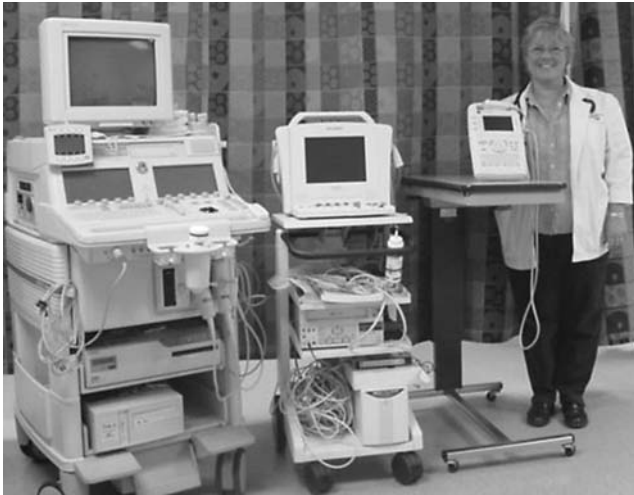
Figure 3. Picture showing various types of ultrasound systems. At left a large “full-size” system is shown that can perform all types of imaging. At center is a miniaturized system that has most of the features of the full service system, but limited display, analysis and recording formats are available. The smallest “hand-held” system shown at right has basic features and is battery operated. It is designed for rapid screening exams integrated into a clinical assessment at the bedside, clinic, or emergency room.
