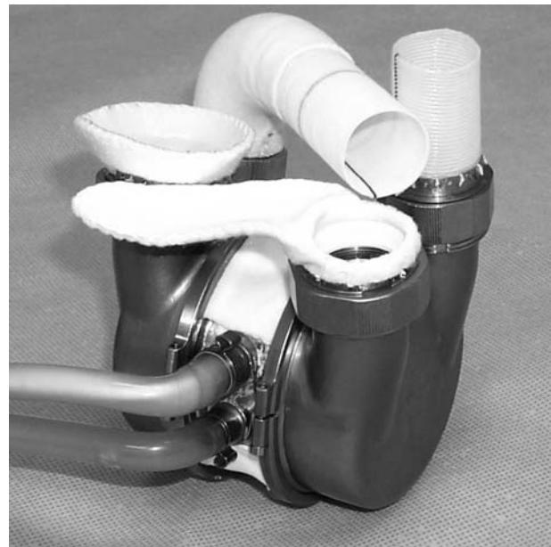
Figure 17. Penn State/3M Electric Total Artificial Heart. This artificial heart is composed of two blood pumps that are of similar design to the Penn State/Arrow electric ventricular assist device. However, the electric TAH uses a single implantable energy converter that alternately drives each ventricle.
