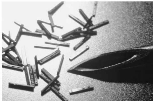
Figure 13. MEMS pressure sensors next to a 30-gauge needle (Courtesy of Silex Microsystems, Jarfalla, Sweden.)
