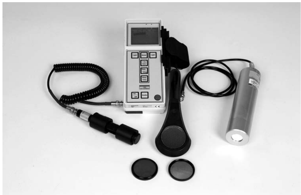
Figure 9. A counter (center; Cardinal Health; Victoreen, Model 190) with an energy-compensated sliding window GM probe (left; Cardinal Health; Inovision, Model 90-12), a pancake detector with filters (center; Cardinal Health; Inovision, Model 489-118FS), and a 1 × 1 in. NaI(Tl) detector (right; Cardinal Health; Inovision, Model 425-110).
