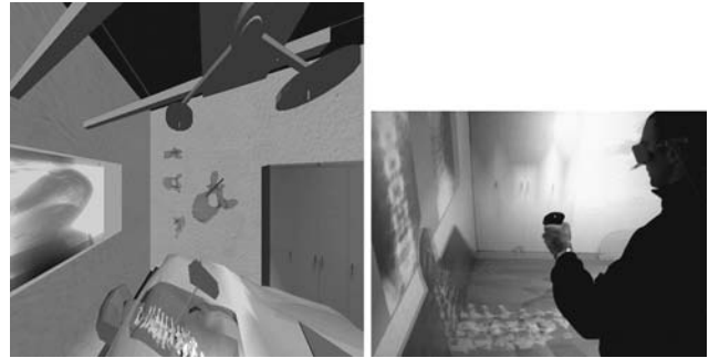
Figure 16. Virtual reality spine surgery simulator. The left panel shows one part of the virtual surgery room with the operating table, the patient and the exposed spine, as well as the radiographs and a magnification of the selected vertebra. The right panel shows an operator that is performing a virtual reality surgery (using stereo stereoscopic glasses and a 3D mouse).
