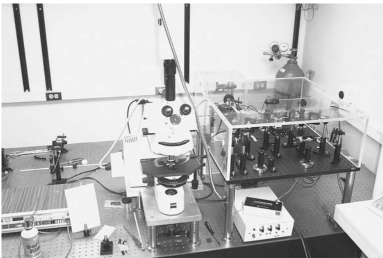
Figure 3. Photograph of an optical tweezers instrument. Note the vibration isolation table that prevents spurious vibrations from affecting experiments. The clear plastic cover minimizes ambient air convection that might affect the laser path in addition to limiting access of dust and preventing accidental contact with the optics.
