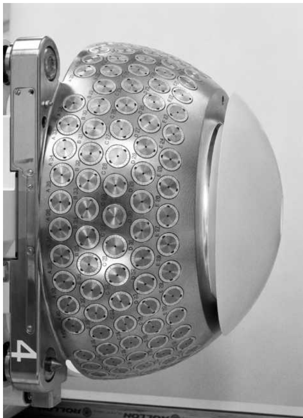
Figure 6. (Upper panel) Collimator helmets for Leksell Gamma Unit Model U. (Lower panel) Collimator helmet for Leksell Gamma Unit Models B and C.
