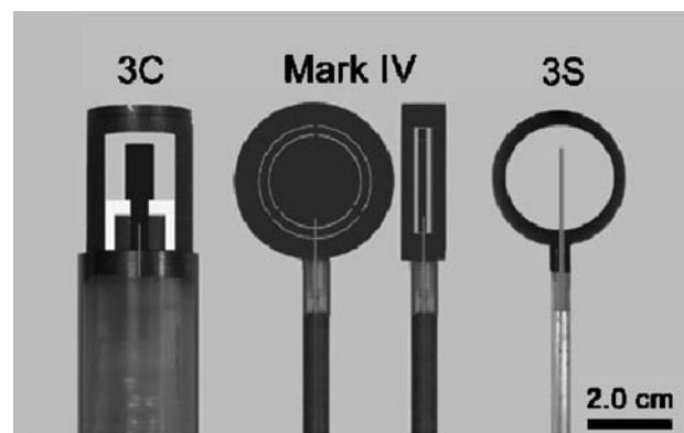
Figure 2. Schematics of three graphite-walled cavity ion chambers designed and operated at the National Research Council (NRC) - cylindrical (3C), parallel-plate (Mark IV), and spherical (3S). The 3S utilizes an aluminum electrode, while the other two chambers utilize graphite electrode.
