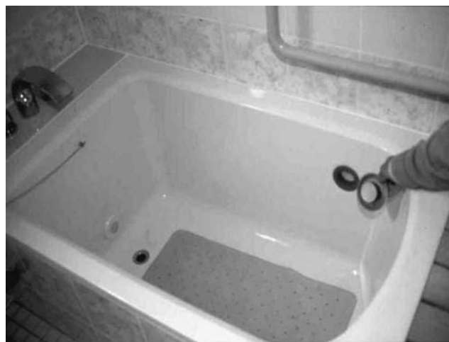
Figure 7. The ECG recorded from a bathtub. Silver–silver chloride electrodes are placed in the bathtub and the ECG signal can be obtained through the water.
