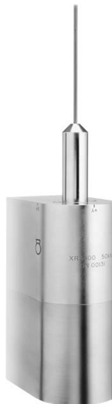
Figure 13. INTRABEAM X-ray tube. The body of the device contains the high voltage electronics, power for the steering coils and the electron gun. It also contains the internal radiation monitor for integrating the radiation output of the device, similar to the internal ionization chambers in a linear accelerator. Electrons are accelerated to the tip of the probe where they strike a gold target and produce the X rays. The large diameter section contains the steering coils.
