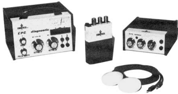
Figure 6. This represents one of the earliest families of stimulators, with the original model seen on the left . The first personal patient treatment model is depicted on the right , and a prototype for a miniaturized design is shown in the center . The original sponge electrodes are depicted in the foreground .
