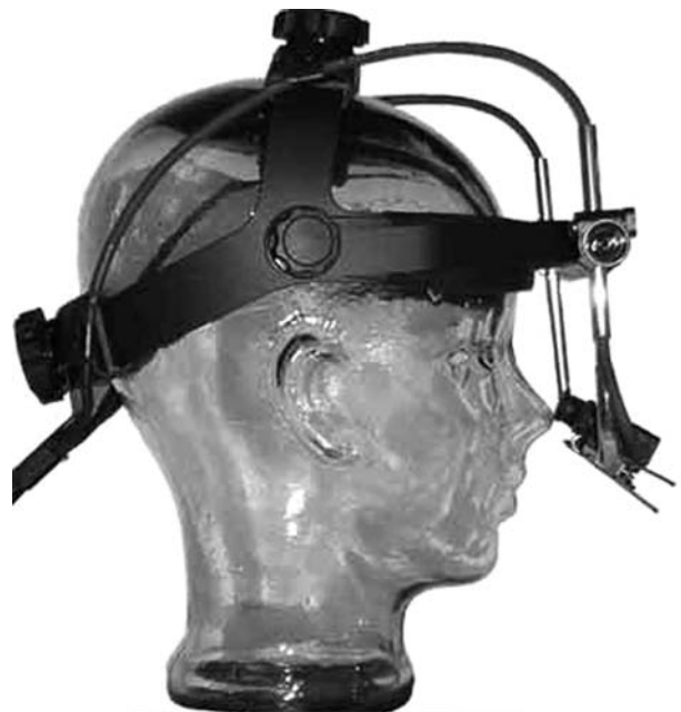
Figure 18. Head mounted camera and illuminator module is mounted on a stalk, and is aimed directly at the eye. (Courtesy of SR Research, Inc. Ontario.)
