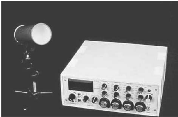
Figure 3. A “mini-Ganzfeld” based on light emitting diode technology. The device shown has four independent color channels, blue, green, orange and red, each of which can be used as stimulus or background alone or in combination. (Courtesy of Chris Hogg, CH electronics, Bromley, Kent, UK; www.ch-electronics.net.)
