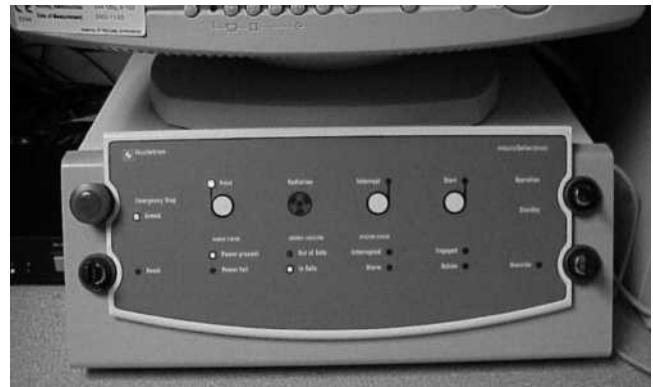
Figure 13. The Treatment Control Panel of the Nucletron, micro-Selectron HDR RAL. The START button is the white button on the right side of the panel, while the EMERGENCY OFF button is the top button on the left side of the panel.
