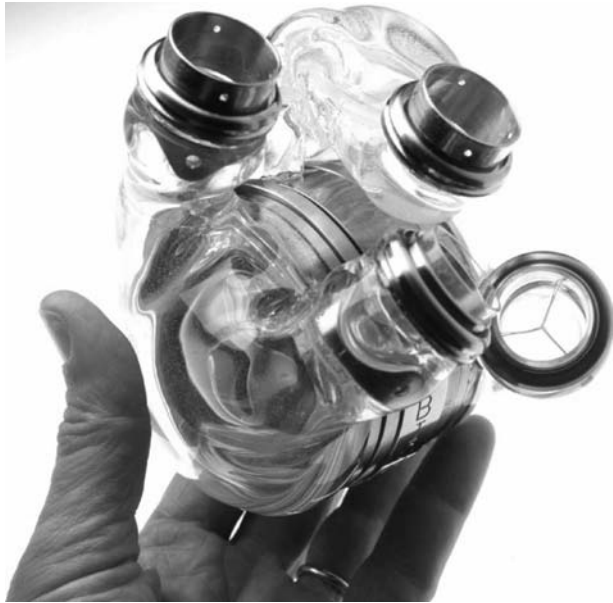
Figure 18. ABIOMED AbioCor Electric Total Artificial Heart. The AbioCor TAH uses an electro hydraulic energy converter to alternately compress each blood sac. The AbioCor is currently undergoing clinical trials in the United States. Two patients were discharged from the hospital, with one patient surviving for > 1 year. (Reprinted with permission from ABIOMED, Inc.)
