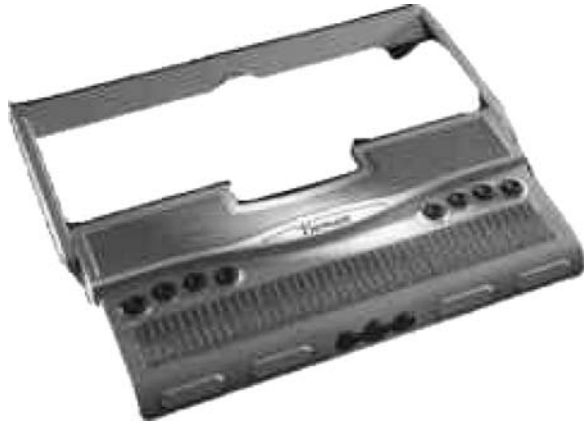
Figure 4. The Braille Voyager 44 made by Manufacturer: F.J. Tieman BV. It has a 44 cell Braille display and 5 navigation keys.
