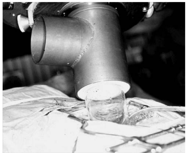
Figure 2. Example of electron beam alignment using the hard docking process. The linear accelerator is a conventional machine in the therapy department and the applicator was fabricated in-house.
