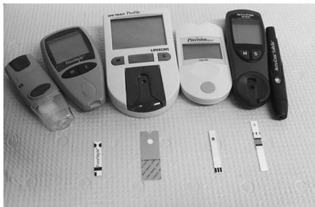
Figure 3. A small collection of home glucose monitoring equipment developed over the past decade. At either end (above) are devices used to puncture the skin for sample collection. Examples of commercial glucose meter (above, center) are also shown. Strips (below) contain immobilized glucose oxidase and are discarded after a single measurement.
