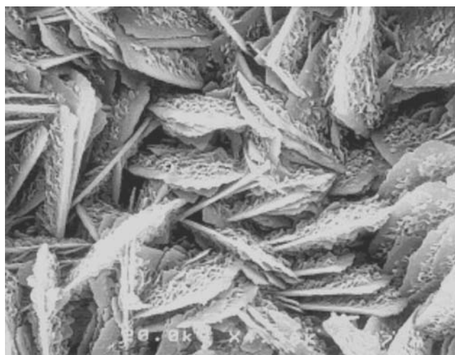
Figure 20. The SEM photograph showing the surface morphology of the SHA700 immersed in SBF for 1 week.
