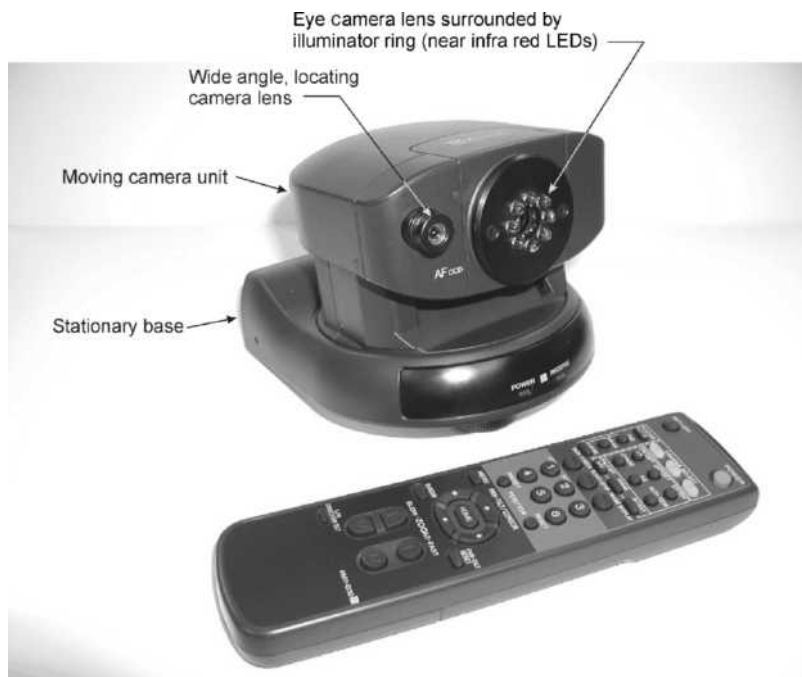
Figure 19. Example of a remote eye tracker optics module that moves in azimuth (pan) and elevation (tilt) to keep a telephoto eye image within the camera field of view. (Courtesy of Applied Science Laboratories, Bedford, MA.)
