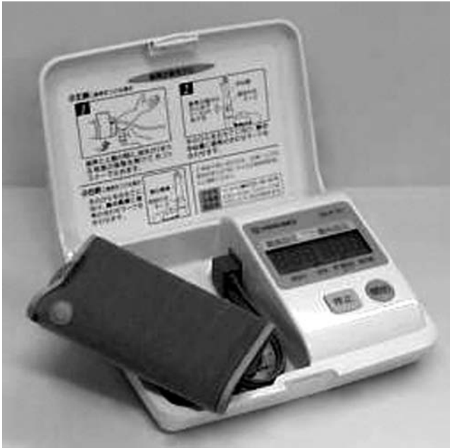
Figure 2. Automatic blood pressure monitor using both auscultatory and oscillometric methods.
