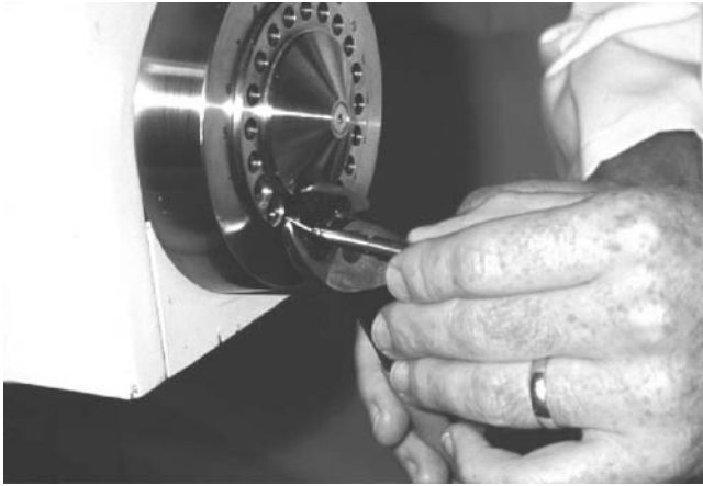
Figure 17. Cutting the source cable from a treatment unit. This procedure should only be performed in very special, rare situations as described in the text. Great care must be taken to assure the cut is through the cable and not the source capsule.
