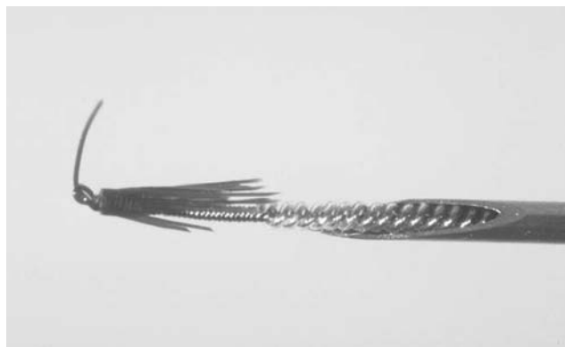
Figure 7. A "Peterson" type intramuscular electrode design. This is a helically wound PFS insulated multistranded 316LVM stainless steel wire design that is attached to a barb-like anchoring structure constructed of polypropylene suture material. The wound section of the electrode is \sim 800\ \mu\text{m} in diameter and is partially loaded into a hypodermic needle. (Courtesy of J.T. Mortimer and reproduced by permission of World Scientific Publishing Co.)
