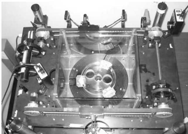
Figure 8. An optical scanner developed for use with polymer gels. (Photograph by M. Heard.)
