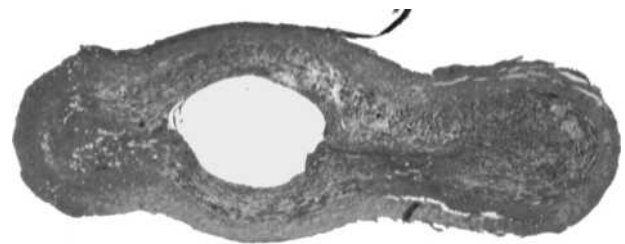
Figure 18. Histologic cross-section of a vessel sealing experiment in the canine femoral artery. Successful seal obtained with a center temperature of 89 °C for 2 s. Hole in center of section is location of thermocouple used to monitor temperature. Original magnification 40x.
