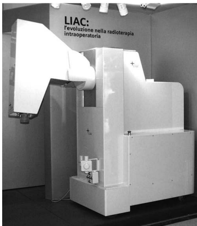
Figure 7. Liac mobile linear accelerator by Info&Tech. This unit looks similar to the Novac7 in terms of its movements and clinical set up, but there are differences in the design (see text for details).
