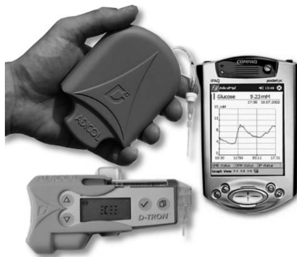
Figure 2. Components used by the Adicol’s biomechanical artificial pancreas. Top left corner shows the microperfusion probe connected to the glucose monitor, which includes microfluidics components, Bluetooth communication, and the sensor. The handheld iPAQ PocketPC maintains wireless communication with the other two components, runs the MPC controller. Disetronic D-Tron insulin pump is equipped with a special sleeve visible on the left hand side of the pump which converts the Bluetooth radiofrequency signal to an infrared signal accepted by the pump (reprinted with permission from (54)).
