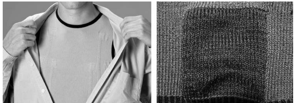
Figure 27. (a) The WEALTHY physiological monitoring vest with integrated sensors. (b) An early version of the fabric electrodes.
