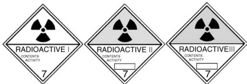
Figure 3. Labels for radioactive packages based on the activity contents and radiation levels outside as given in Table 15.
