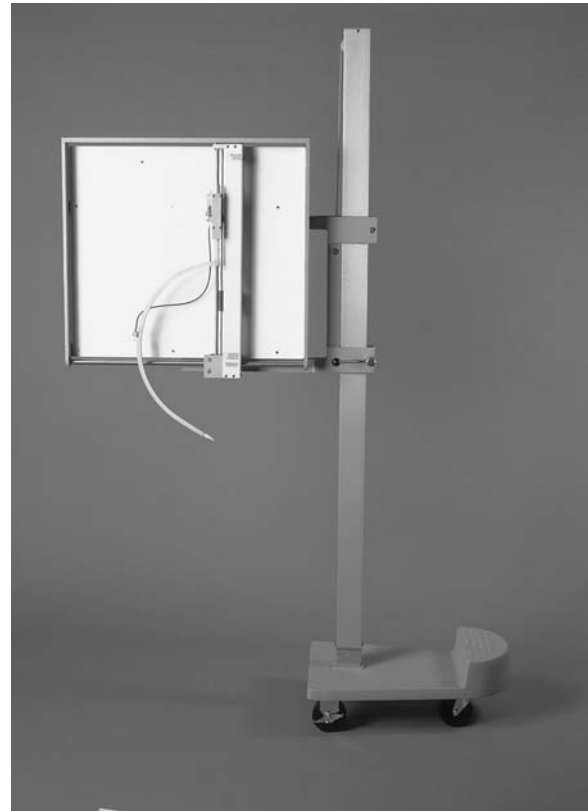
Figure 4. Contour plotter. The device is a simple, easy-to-use precision pantograph that links a drawing pen to a stylus arm and, upon contact with the body, communicates body contours to an overhead drawing board. The contour plotter is suspended on a vertical column and can easily be adjusted and locked securely. A continuous plot is drawn as the operator follows the physical contours of the patient. Marks can be made along the contour to indicate beam entry and laser light locations. (Courtesy of MEDTEC.)
