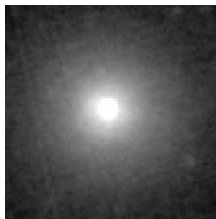
Figure 9. The OCT image of a polymer gel exposed to an ^{192}\text{Ir} HDR brachytherapy source. The central region was occupied by the source during irradiation and was replaced with irradiated gel for imaging (117).
