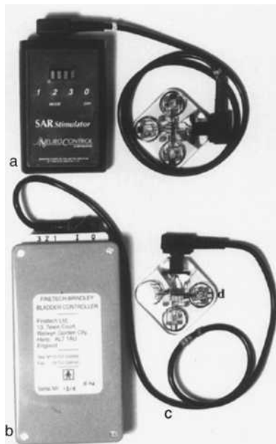
Figure 25. External equipment. (a) New control box. (b) Original control box. (c) Transmitter lead. (d) Transmitter block.
