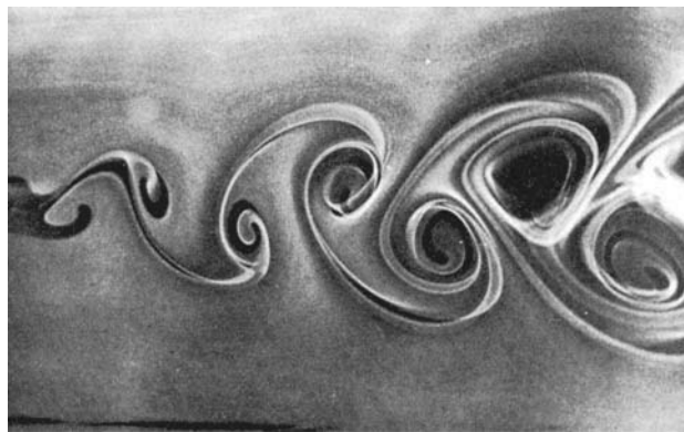
Figure 7. Vortex shedding from a circular cylinder. Picture from White (23), courtesy of the U.S. Naval Research Laboratory.
