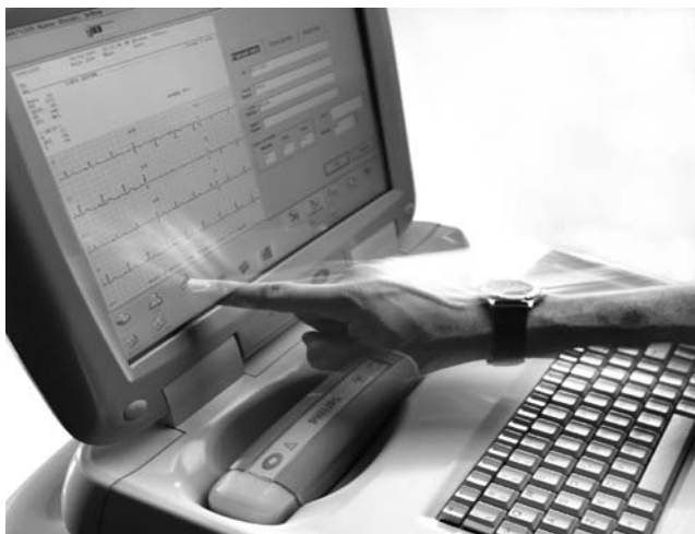
Figure 9. PageWriter Touch, a high-end 12-lead electrocardiograph with built-in 12-lead ECG signal interpretation capabilities. (Courtesy of Philips Medical Systems, USA.)
