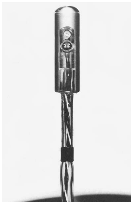
Figure 1. Vaginal photoplethysmograph similar to that originally designed by Sintchak and Geer (3) using a single light source and photodetector. (Courtesy of Farrall Instruments, Inc., Grand Island, NE.)
