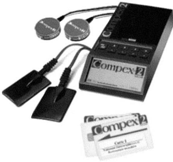
Figure 4. The Compex Motion FES system, manufactured by the Swiss based company Compex SA, is a general purpose programmable transcutaneous electrical stimulation device. Seen are the stimulator unit, three memory chip-cards that are inserted into the stimulator and used to store all pertinent information for a specific protocol, two EMG sensors, and two surface electrodes. (Reprinted from Ref. 83 with permission from the Institute of Physics and Engineering in Medicine.)
