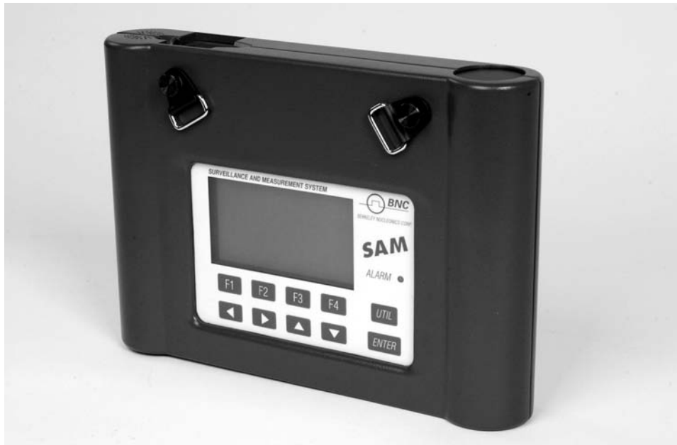
Figure 15. A portable NaI(Tl) surveillance and measurement (spectroscopy) system. (Berkeley Nucleonics Corp., SAM Model 935).
