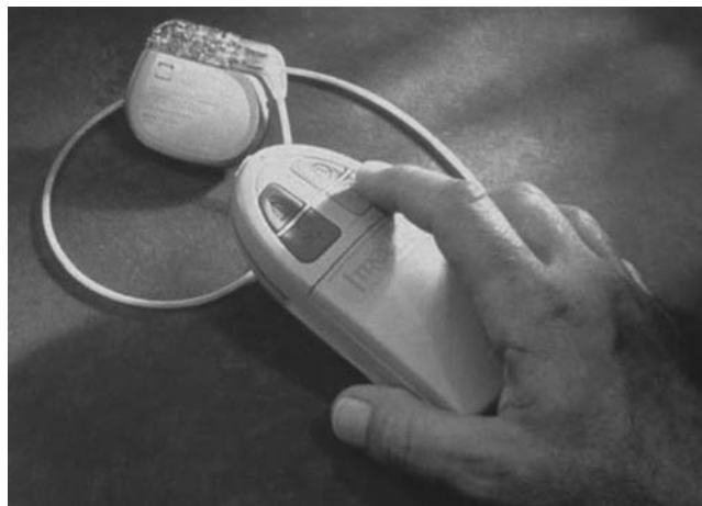
Figure 5. Implantable IPG with hand-held controller. (Used courtesy of Medtronic, Inc.)
