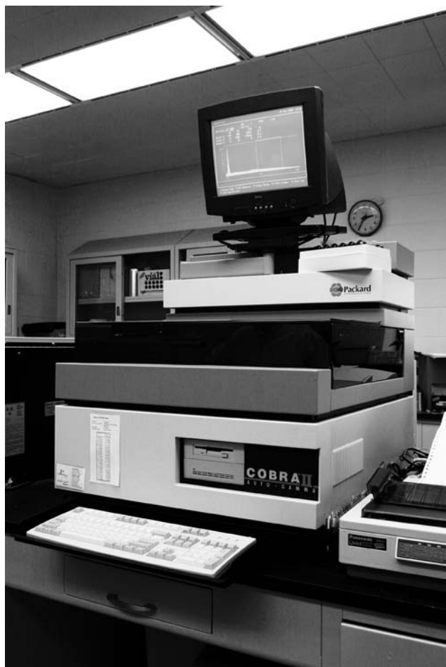
Figure 11. A \gamma -counter system with a 1 × 1 in. (2.54 cm) NaI(Tl) detector to identify and measure \gamma rays. (Canberra; Packard, Model Cobra II Auto-Gamma.)
