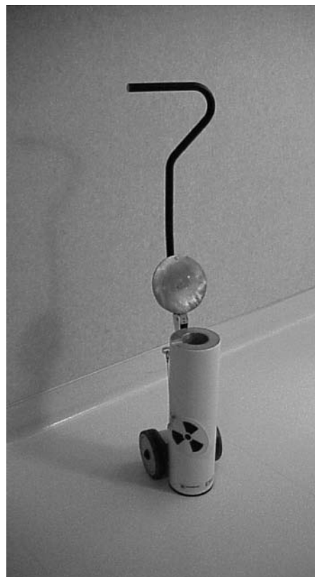
Figure 16. The shielded container for emergency placement of an unretracted source.
