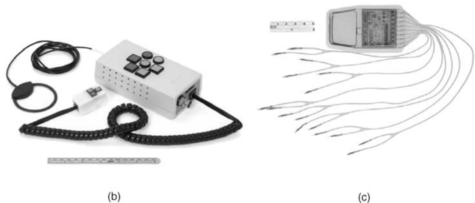
Figure 3. (a) Diagram of components for the implanted stimulation system developed at the Cleveland FES Center and commercialized as the Freehand neuroprosthesis by NeuroControl Corp. In the hand-grasp example shown, shoulder position is transduced for use as the command input. (b) The external control unit (ECU) provides the transducer interface, user control algorithm, multichannel stimulus coordination, and power for the implanted receiver-stimulator system. (c) The implanted receiver-stimulator provides multiple channels of stimulus output via the leads seen in the figure. It also transmits implantable sensor data to the ECU, and is powered through an inductive link that forms a coreless bidirectional transformer. Intramuscular or epimysial electrodes implanted in the forearm or hand are attached to the stimulator leads (not shown). (Courtesy of the Cleveland FES Center.)
