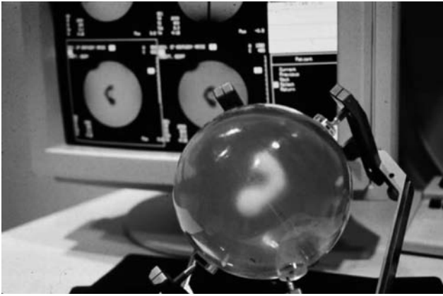
Figure 12. A BANG gel irradiated with a highly conformal dose distribution produced by a Gammaknife treatment unit. The distribution can be appreciated qualitatively without the need of imaging systems or processing. (Photograph by the author. See also Ref. 161.)
