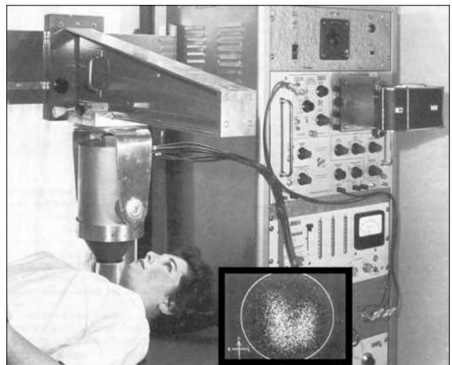
Figure 3. Initial Anger camera used to image a patient's thyroid with I-131. The field of view of this device was 10 cm. (Reprinted from Seminars in Nuclear Medicine, Vol 9, Powell MR, H.O. Anger and his work at Donner Laboratory, 164-168., 1979, with permission from Elsevier.)
