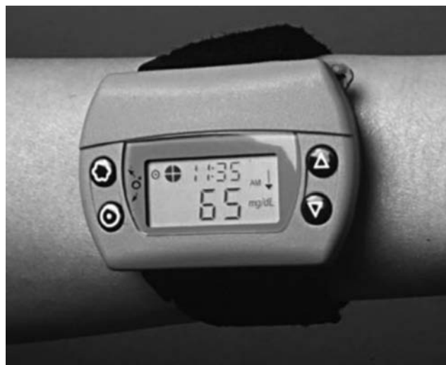
Figure 5. The Glucowatch Biographer (43). An integrated system for sample extraction by reverse iontophoresis and glucose sensing. (Used with permission from John Wiley & Sons, Inc.)
