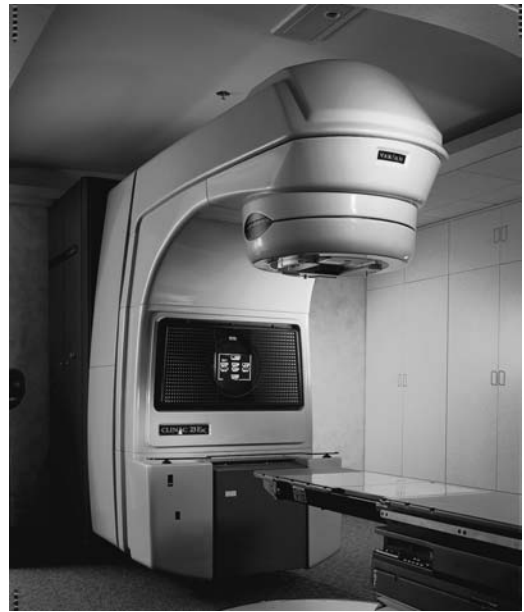
Figure 3. New generation radiation therapy simulator, in which image intensifier system has been replaced with amorphous silicon flat-panel that produces high resolution, distortion-free images and facilitates a filmless department. (Courtesy of Varian Medical Systems.)
