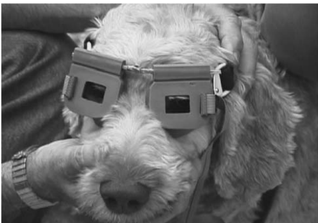
Figure 4. IR system to measure the horizontal and vertical eye movements of both eyes shown mounted in goggles for a human subject (a) and a canine subject (b).
