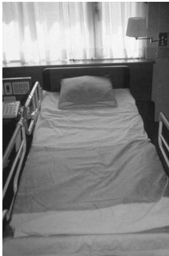
Figure 6. The ECG recorded from the bed. Electrodes are placed on the pillow and the lower part of the bed. An ECG signal can be obtained during sleep.
