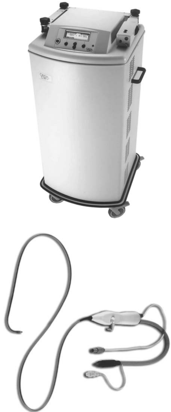
Figure 4. Modern cryosurgical device, cooled by nitrous oxide, used in cardiac cryosurgery for the treatment of atrial fibrillation and other arrhythmias. The console houses the primary gas supply in cylinders, the gas circuits, and the controlling electronics and software. The device cools the catheter probe by passing the pressurized gas through a restricting orifice at the probe tip. The probe is a steerable cryoablation catheter with leads to connect to the console for cryogenic gas flow, pressure monitoring at the catheter tip, and cardiac electrical signal recording (Fig. 3b). (Photographs by courtesy of CryoCor Inc., San Diego, CA 92121.)
