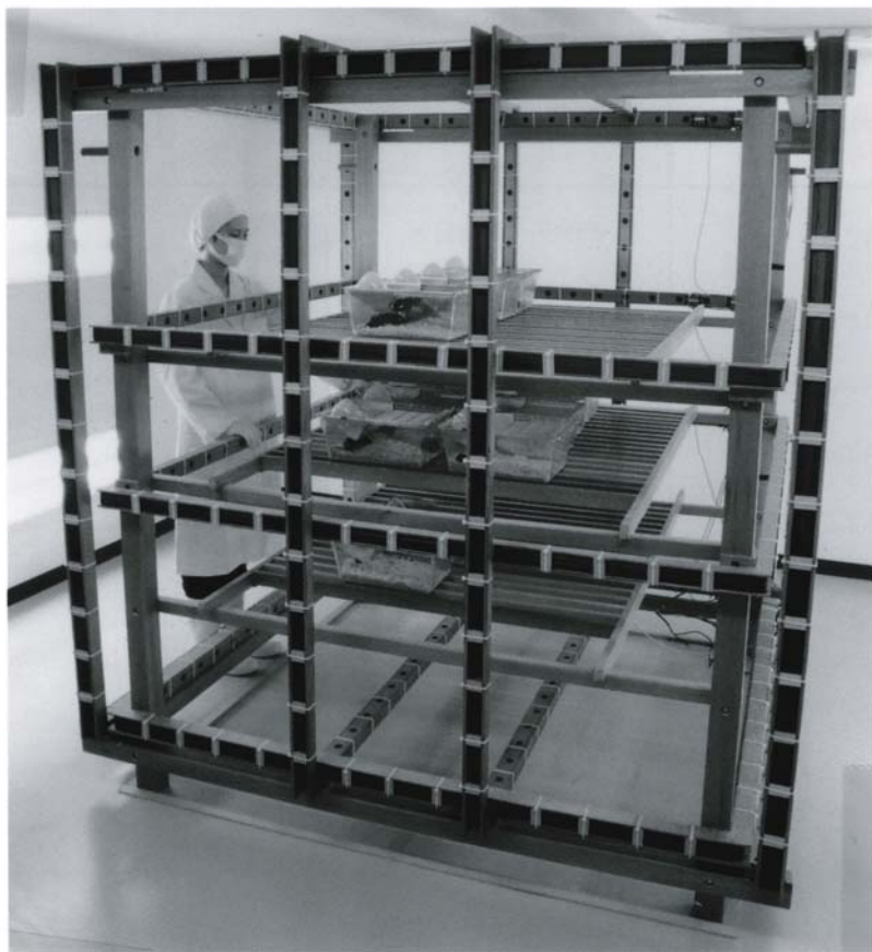
Fig. 5.3. The newly developed magnetic field exposure system for in vivo experiments.
