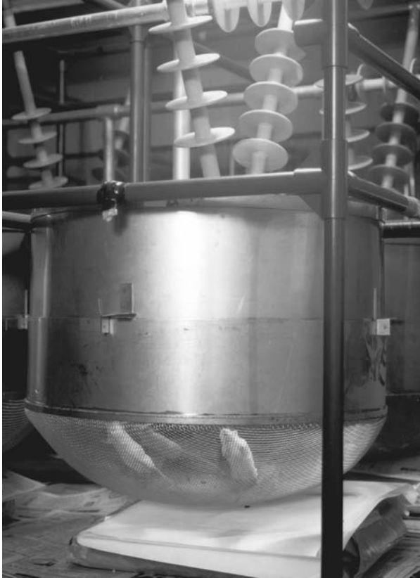
Fig. 5.2. An improved electric field exposure system for experiments with small animals, such as mice and rats.
