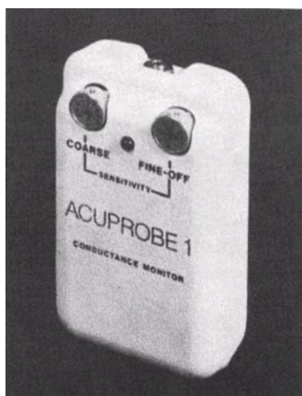
Figure 2-25. The Acuprobe I-a small, hand-held, unit for point location by skin conductance measurement, capable of sensing with very low currents in the region of 0.5-1.0 microamperes. Indication is by means of an audible sound plus a visual red light output. Probe-sensing is adjustable by means of two sensitivity controls, coarse and fine, for a full range of skin resistances. The power source is a standard 9-volt transistors battery. (Courtesy of Intertronic Systems, Ltd., Ontario, Canada.)
