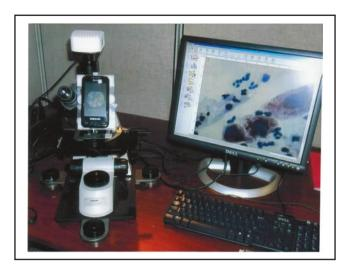
Fig. 7.13 MarkPap mobile image acquisition workstation
