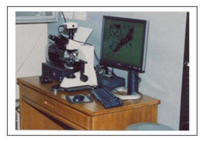
Fig. 7.11 A digital telecytopathology workstation consisting of a microscope, digital camera and computer capture, store and forward image files
