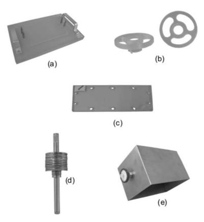
Fig. 23.1. Different parts of the custom-built loading device: The bottom plate of the loading device in which the 6-well plate perfectly fits (a). Two position rings of which one is placed at the top of a cell culture insert (b). The lid for vertical positioning of the indenters (c). Indenters with rings to apply additional weight (d). Lid with air filters to cover the total experimental set-up (e).
