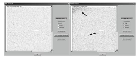
Fig. 15.8. RMAExpress "residuals." A near-perfect microarray is shown on the left. The one on the right shows uneven hybridization and a smudge, arrows.
