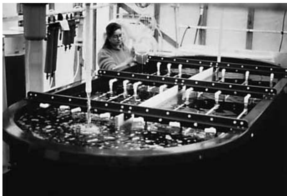
Fig. 2. One of two prototype 5,000-liter aquaculture growout tanks for B. neritina .
