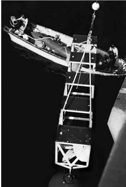
Fig. 3. The 7-m steel prototype in-sea aquaculture structure for B. neritina , showing culture panels, flotation sphere and orientation propeller, being launched from the pier of Scripps Institution of Oceanography, La Jolla, Calif.
