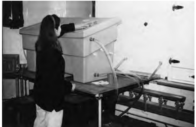
Fig. 2.3 Back in the laboratory: (a) preparation of dinosaur specimens at the Royal Tyrrell Museum of Palaeontology, Drumheller, Alberta, Canada, using a dental drill to remove rock matrix from the bones; (b) Rachael Walker adjusts an automated sieving machine for processing sediment containing microvertebrate remains, designed by David J. Ward, in the Palaeontology Laboratory, University of Bristol, UK. (Photographs by MJB.)
