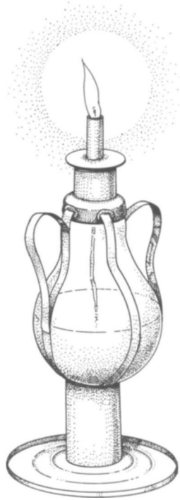
FIGURE 22: An ingenious spirit lamp. People make their own light where electricity does not reach. A light bulb is inverted and used as a reservoir into which a wick dangles. A tin can is cut and fashioned into a base—complete with handles—for the lamp.
