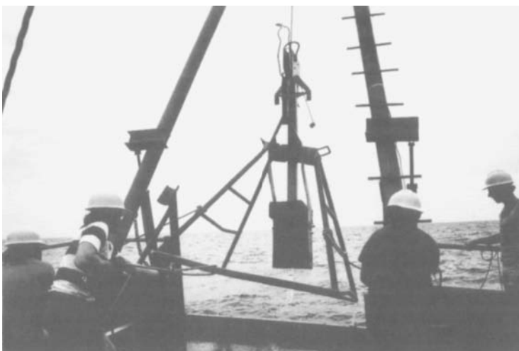
FIGURE 7.6 Box corer. After the frame hits bottom, the coring device is forced into the sediment mechanically. (Courtesy of Sand M)
