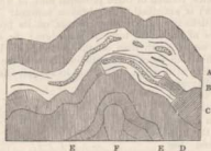
A, D, F. Beds of clay-slate, with cleavage-laminae perpendicular to the horizon. E and part of C. Similar beds, with the cleavage at right angles to every flexure. B and parts of C. Beds of imperfect, non-laminated clay-slate, with intercalated seams of sandstone represented by the dotted parts. F. Nucleus or core of clay-slate formed by the lateral crushing of the strata, about two feet high and one foot broad. These nuclei occur in almost all the folds.
