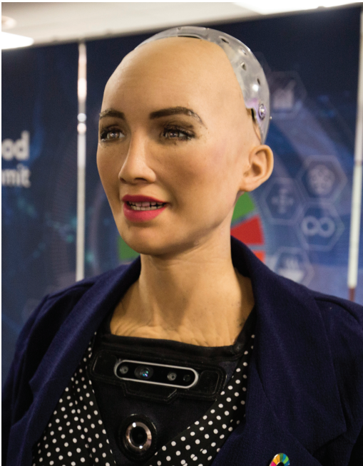
Figure 8.3 Sophia. Sophia, an AI development by Hong Kong-based Hanson Robotics, is currently the most human-like robot. She can simulate human facial expressions and gestures, recognize faces, answer questions, and carry on simple conversations. Sophia is the first robot to have citizenship.
