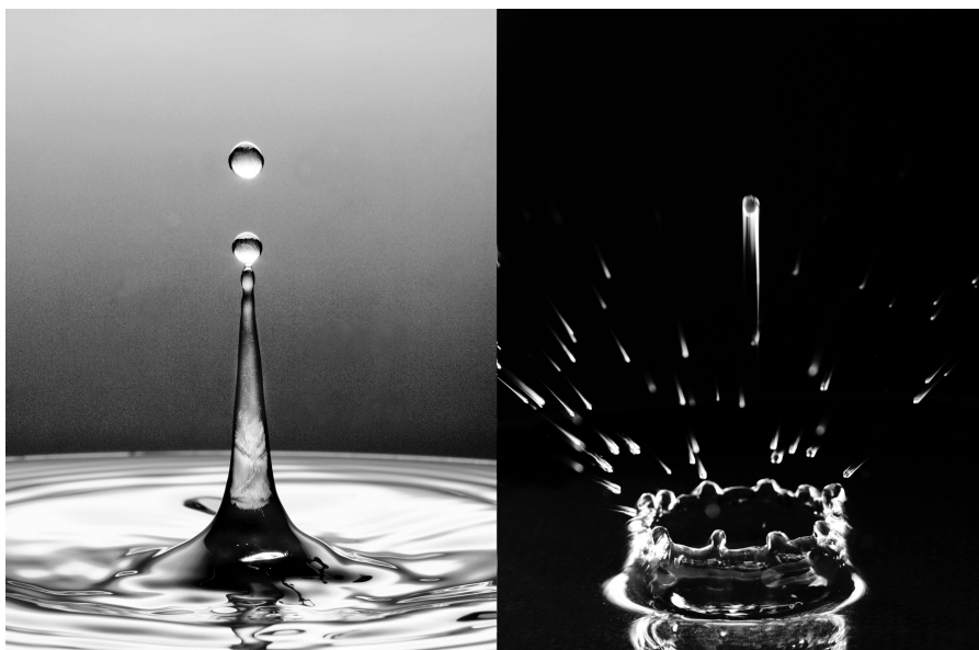
FIGURE 18.2 (See color insert following page 302.) Formation of jet drops and film cap drops from a bursting bubble. Left: For small bubbles (<0.5 mm) surface tension-driven “jet drops” are formed. The material making up successive jet drops from a single bursting bubble comes from successively microtomed layers of its air–water interface (MacIntyre, 1974c). Right: For larger bubbles a very large number of “film cap drops” are produced by a gravitationally-induced instability mediated through the bubble cap’s draining. (Photographs by Prof. Andrew Davidhazy, 2009. With permission.)
