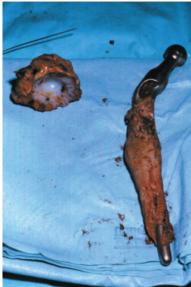
The components of a prosthetic hip joint, removed due to loosening. On the right is the metal shaft encased in the cement which fixed it to the inside of the femur. On the left is the plastic socket. (Custom Medical Stock Photo. Reproduced by permission.)
