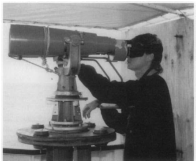
Figure 2 “Big eyes” used to search for marine mammals on large survey vessels. Photograph by Jay Barlow.
