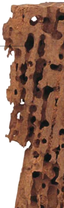
Wooden beam has been attacked by deathwatch beetles
