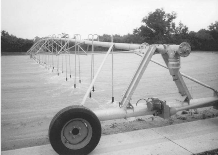
Figure 7.8 An infiltration-percolation system in Pénestin, France.
